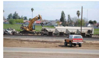
Scrapping this covered hopper car on the spot.
