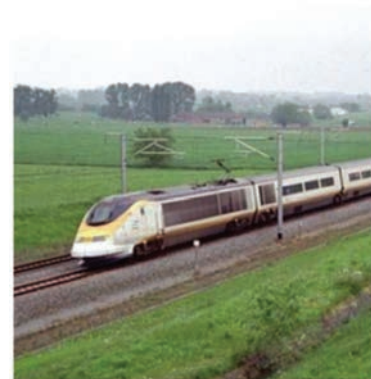
Figure 2-3 Example of an At-grade Profile Showing Catenary Wire System and Vertical Arms of the Pantograph Power Pickups
