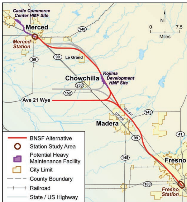
Figure 2-44g BNSF Alternative with Mariposa Way and Le Grand Design Option and Ave 21 Wye
