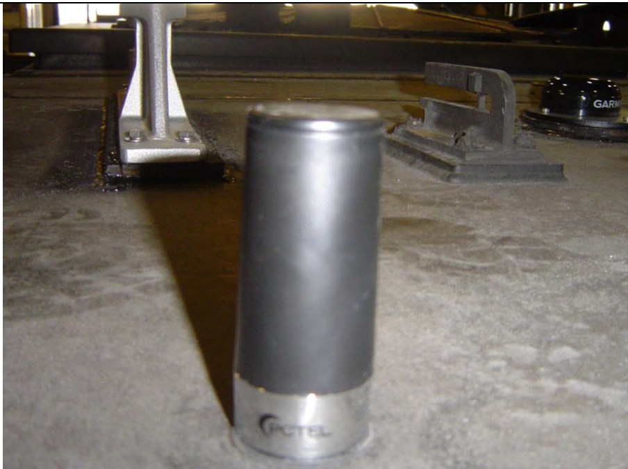
Center antenna is designated as 802.11 According to physical height >3" it can only be in the cellular range Figure 36
