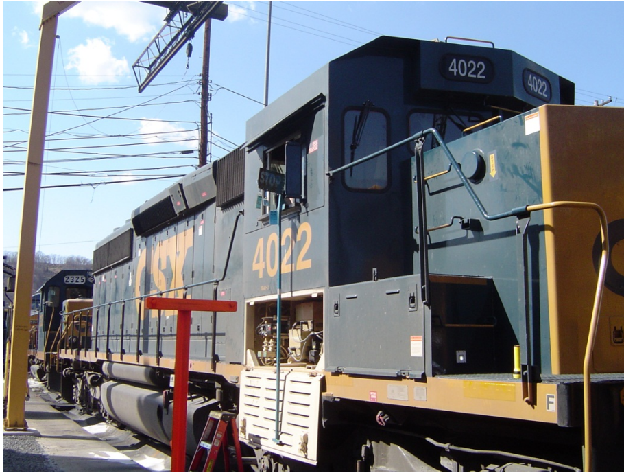
Locomotive under test CSX 4022 SD-40-3 D-E 3000 HP Road Unit Built in 1974 Figure 3
