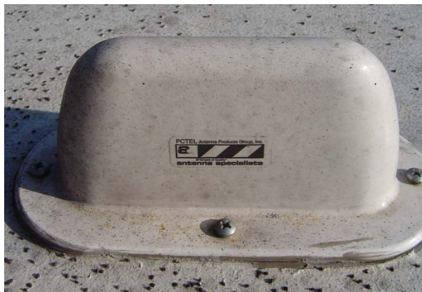
Antenna Specialists ASP 572 UHF Antenna Figure 7
