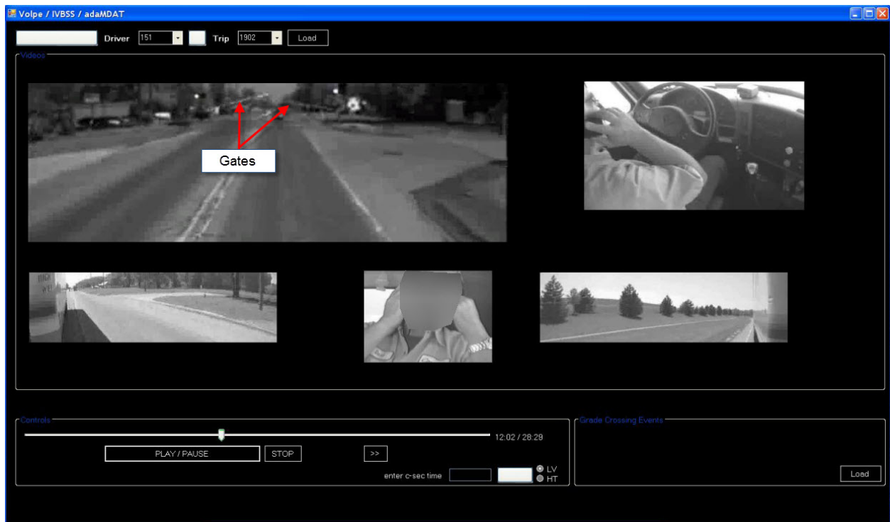
Figure 8. Snapshot of an Event at a Highway-Rail Crossing Equipped with Gates
