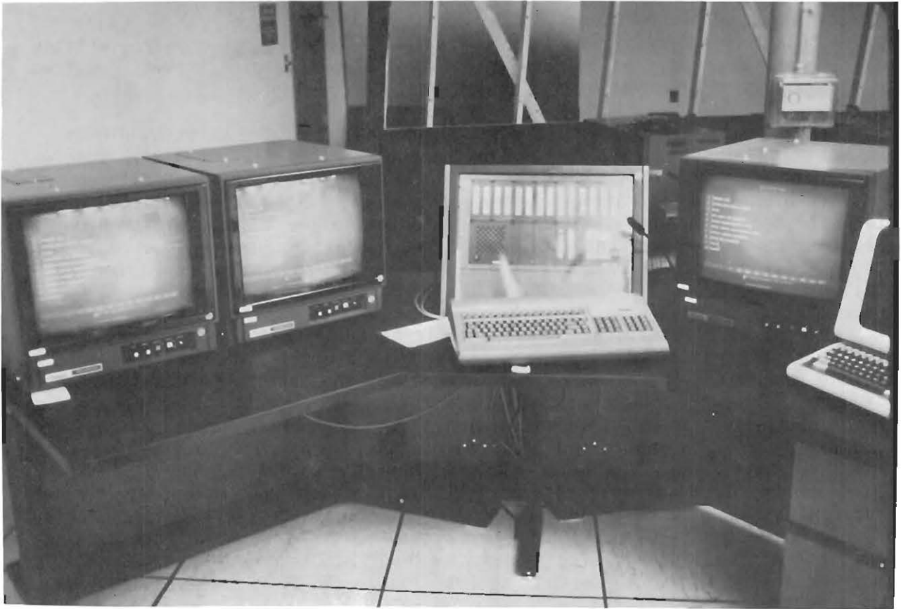
The NEC enters the electronic age . . . Above, CETC control console with touch sensitive control screens and communications panel. Below, track occupancy diagram on projection TV.
