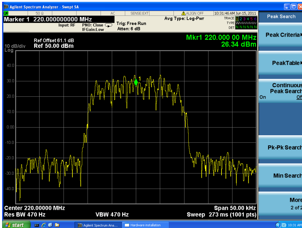
Figure 16: Typical transmission spectrum (DQPSK)
