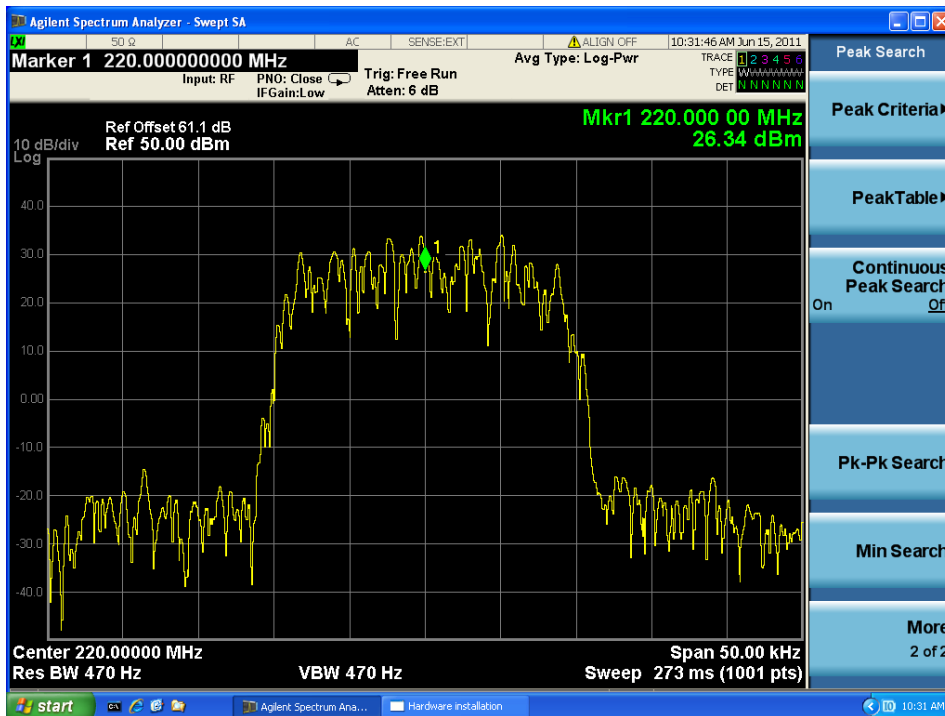
Figure 15: Typical transmission spectrum (DQPSK)
