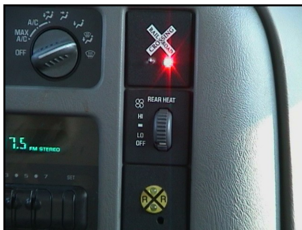
Figure 1. In-Vehicle Highway-Rail Grade Crossing Warning [11]
