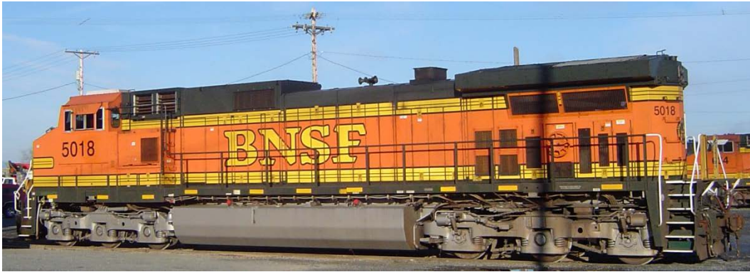
Locomotive under test BNSF 5018 General Electric C44-9W Figure 3
