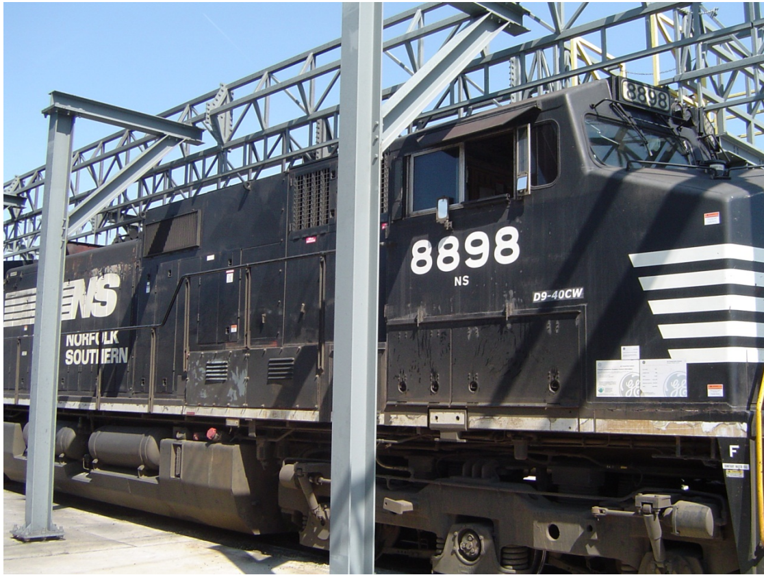
Locomotive under test NS 8898 GE Diesel Electric Locomotive Dash 9-40CW Figure 3
