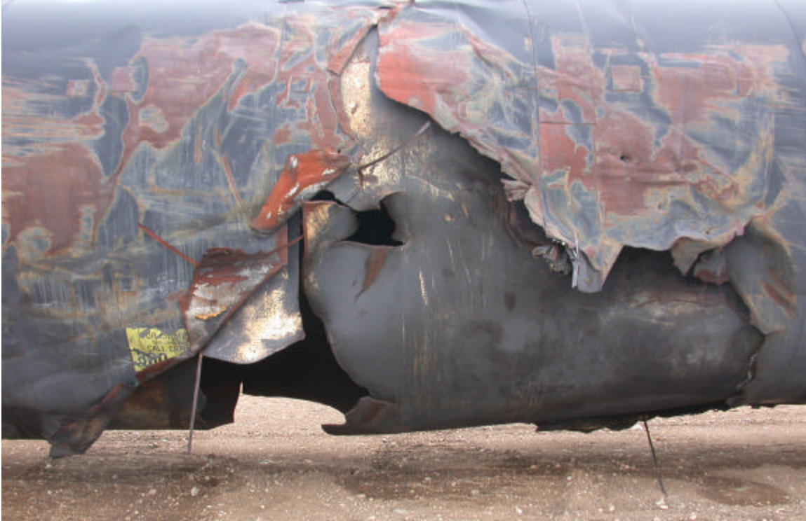
FIGURE 2.24 Puncture and brittle fracture in an anhydrous ammonia tank car that derailed near Minot, ND [1].
