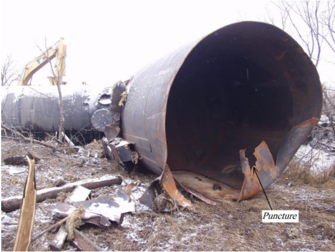
FIGURE 2.26 Puncture and 360-degree shell fracture in an anhydrous ammonia car, which derailed near Minot, ND. Crack propagation from the puncture was by a low-energy ductile fracture mechanism (Fig. 2.14).
