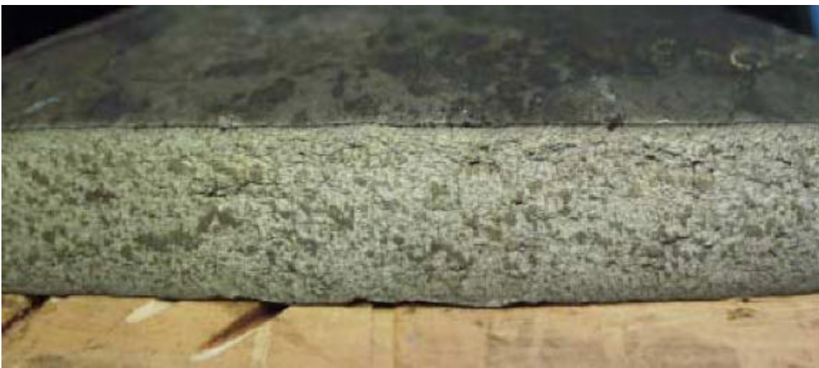
FIGURE 2.8 Ductile fracture in an anhydrous ammonia tank car that derailed near Minot, ND [1].
