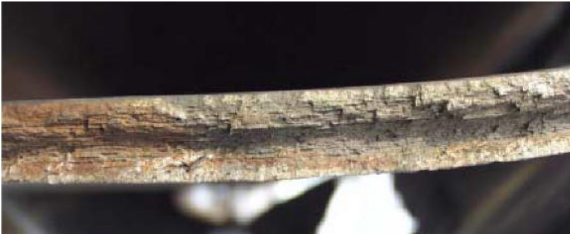
FIGURE 2.14 Low-energy ductile fracture in Minot Car 19 [1]. The fracture propagated in the longitudinal direction, along sulfide stringers, which resulted in a “woody” appearance.
