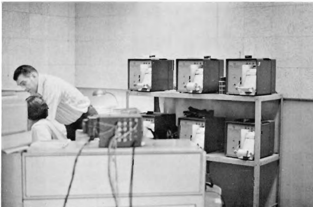
Figure 3-3. Dispatcher's Position with Eight Hot-Box Recorders to Monitor
