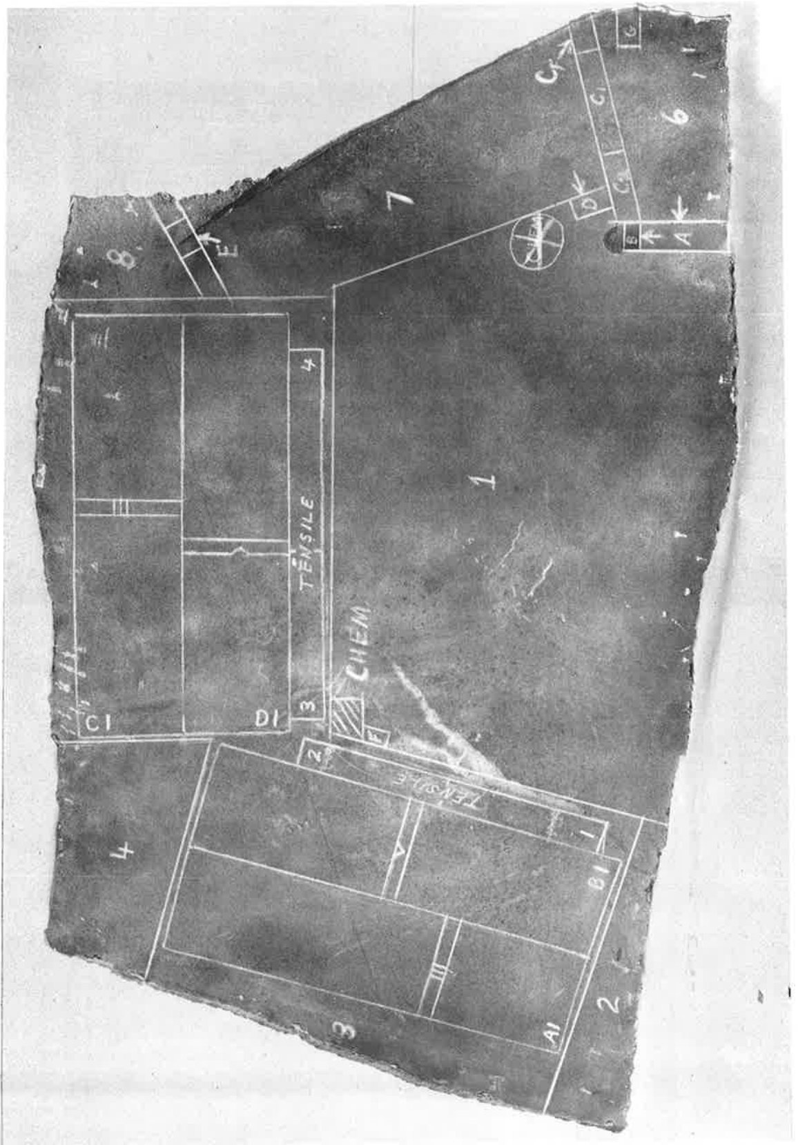
Figure 3. Photograph of the failed plate showing the areas which were used for tensile, impact, and chemical examinations. The metallographic examinations were performed on areas A, B, C 1 , C 2 , C F , D, E, F and G; the hardness tests were also performed on area A. X 1/3
