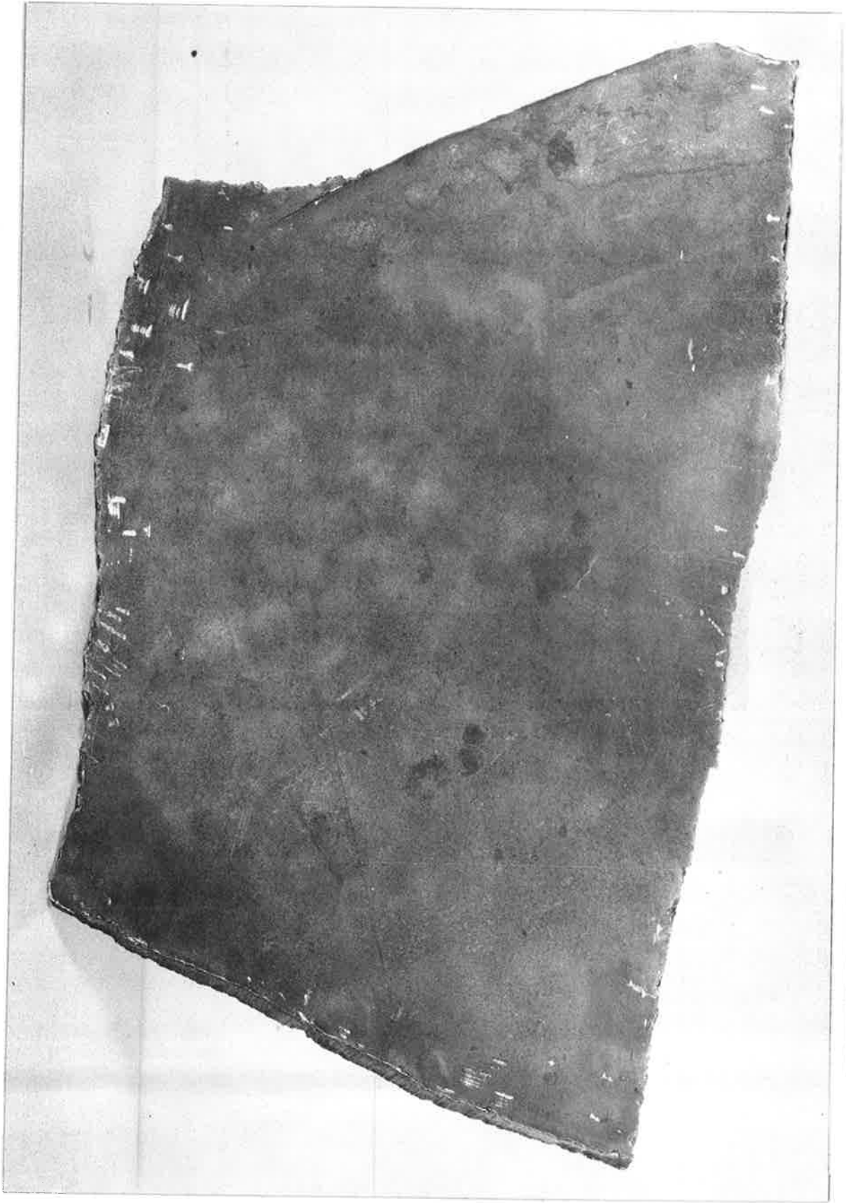
Figure 1. Photograph of the inside of a section of failed tank car plate in the as received condition. Fracture is located at right edge of photograph. X 1/3
