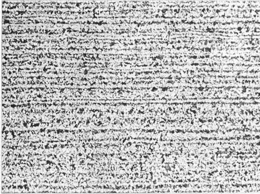
Figure 6. Photomicrograph of the banded structure of the plate. Picral etch. X 100
