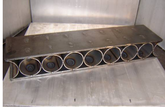
6"x2'x3" Round Tube Core Test Article (P2)
