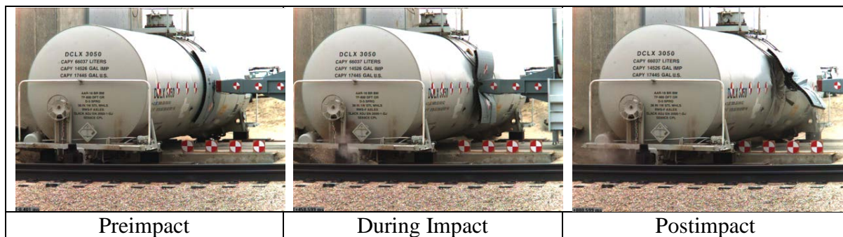
Figure 37. Series of Images Showing Side Impact Progression
