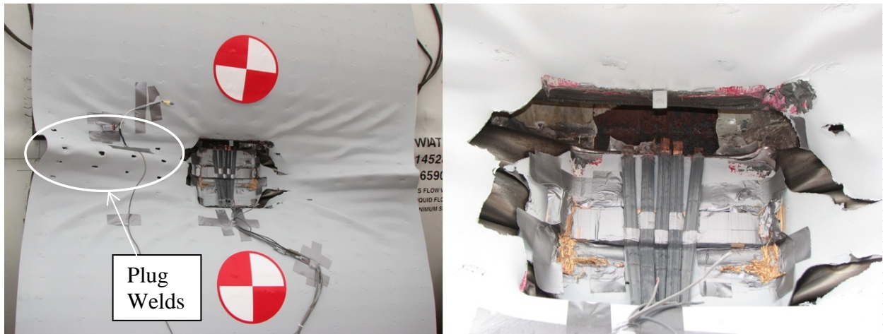
Figure 39. Damage on Protective Panel – Impact Side
