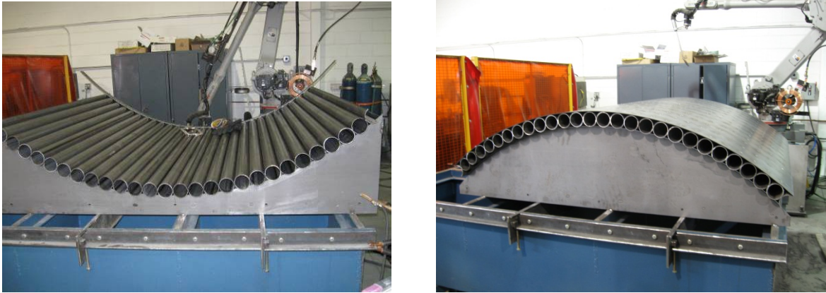
Figure 21. Manufacturing Panel for Impact Test on Concave Fixture (Left) and Convex Fixture (Right)
