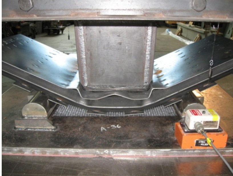
Figure 17. Panel in Three-Point Bend Test with Bubble Wrap to Estimate Load Transfer Area
