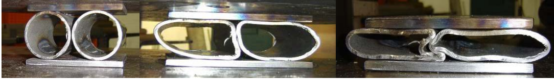
Figure 7. Photos of Round-Tube Panel during Crushing
