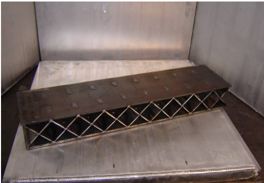
Figure 10. Photos of Manufactured Panels for Uniaxial Compression Tests
