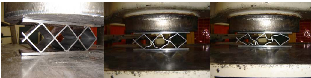
Figure 6. Photos of Diamond Panel during Crushing
