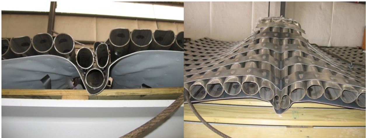
Figure 40. Damage on Protective Panel – Left and Right Sides
