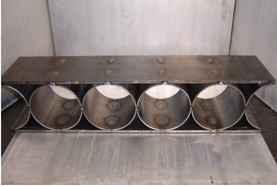
6"x2'x5" Pipe Round Tube Core Test Article (P1)
