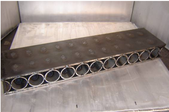
6"x2'x2" Round Tube Core Test Article (P3)
