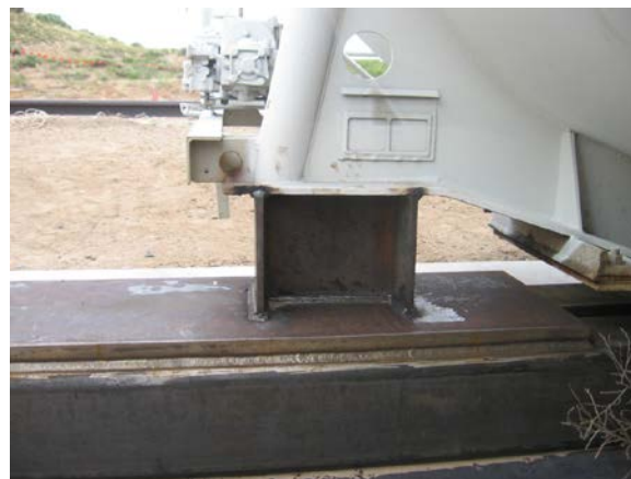
Figure 27. Welded Beam Connecting the Tank Car to the Skid System
