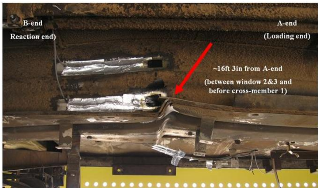
Figure 34. Center Sill Crippling
