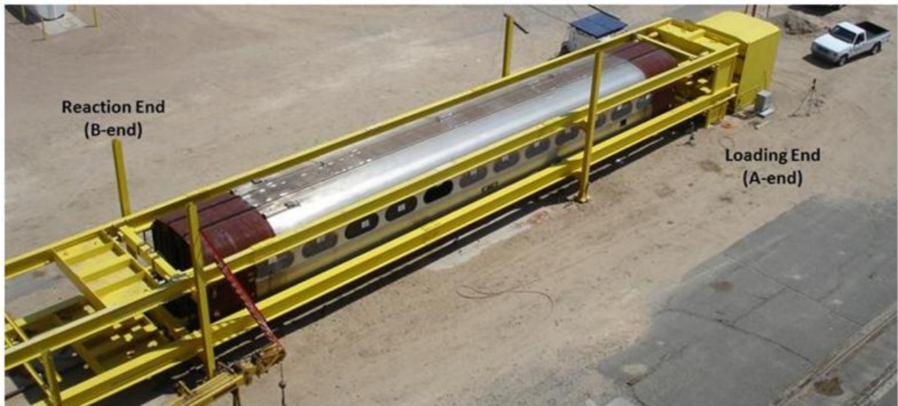
Figure 13. Car 244 in Test Fixture for Crippling Load Test
