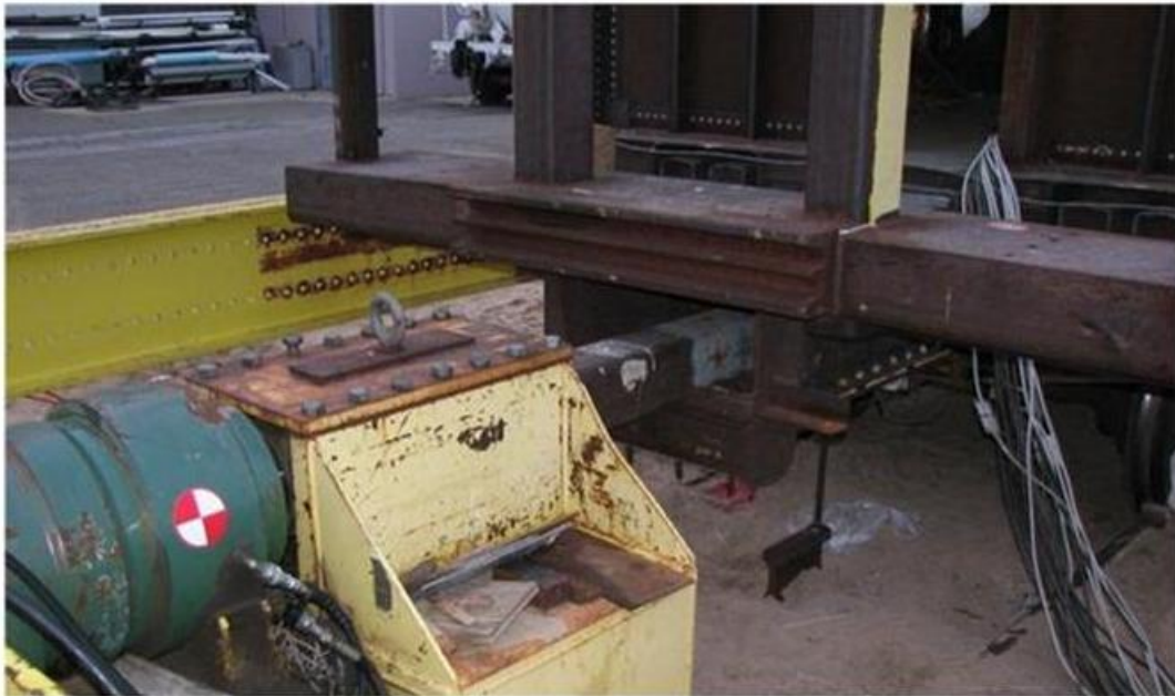
Figure 2. Line-of-Draft Load Applied at A-End for Test 1
