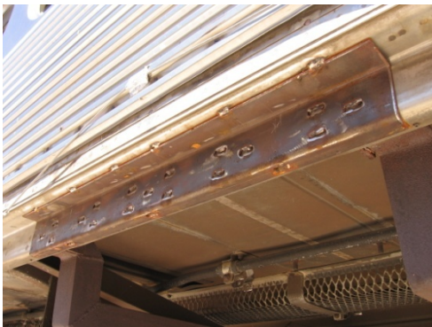
Figure 6. Steel Patch Welded onto Both Side Sills on Car 244
