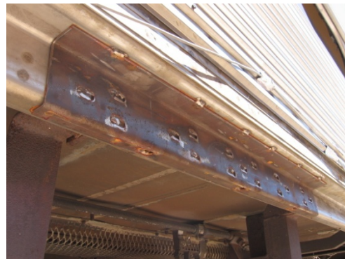
Figure 6. Steel Patch Welded onto Both Side Sills on Car 244
