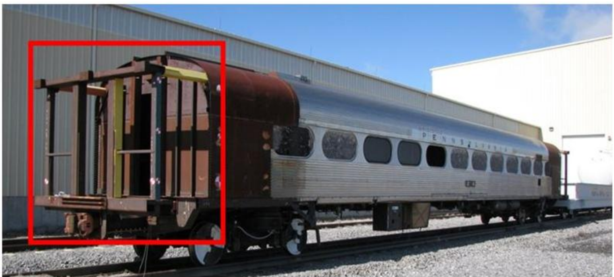
Figure 14. CEM System before Removal for Crippling Load Test
