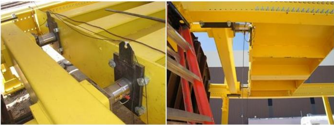
Figure 25. Reaction End Load Cells at Floor and Roof Levels
