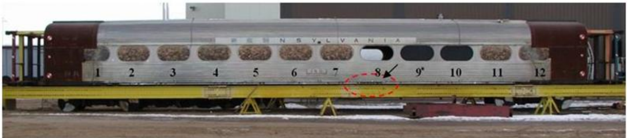
Figure 7. Location of the Steel Patch below Window 8 on Car 244
