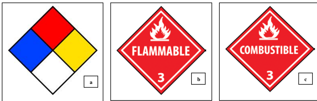
Figure 8. (a) NFPA Diamond Placard; (b) Hazard Class 3 Flammable; and (c) Combustible Placards
