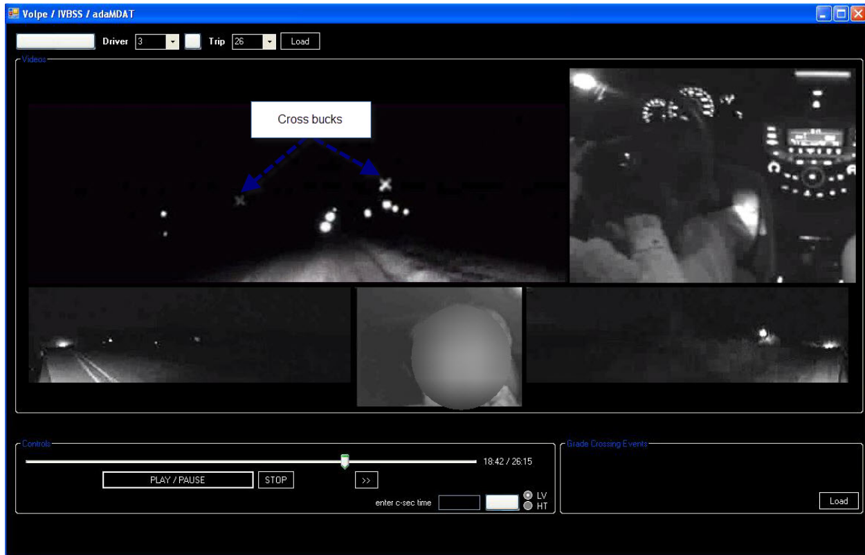
Figure 9. Snapshot of a Grade Crossing Event at a Highway-Rail Crossing Equipped with Crossbucks Only
