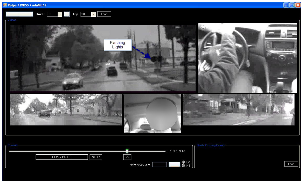
Figure 8. Snapshot of a Grade Crossing Event at a Highway-Rail Crossing Equipped with Flashing Lights
