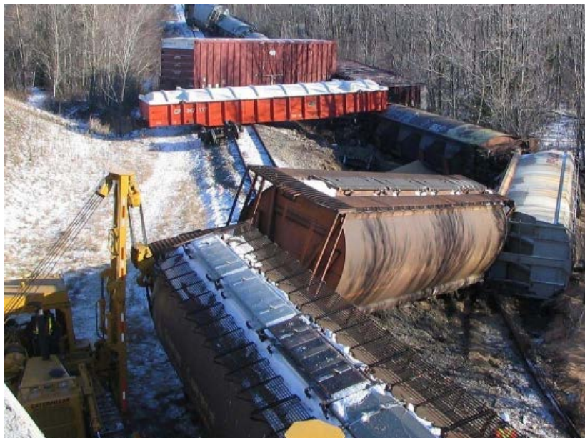
Figure 2.10. Derailed railcar lateral displacement due to embankment
