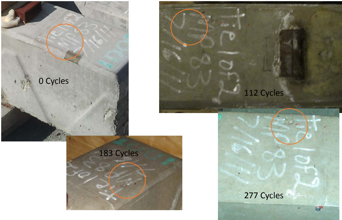
Figure A-25: Tie #1-05009-3 Plant C visual observations.
