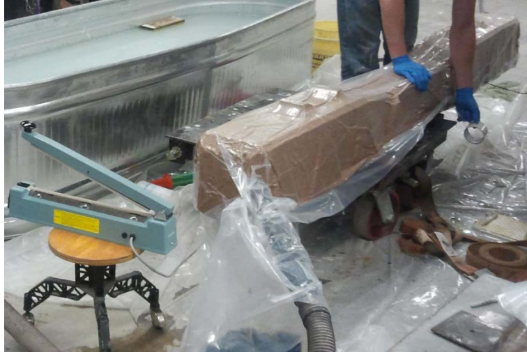
Figure 4: Railroad tie vacuum sealed and wrapped with packing tape.
