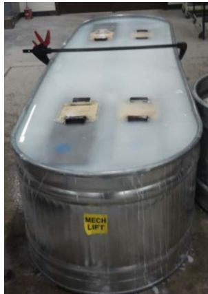
Figure 3: Railroad tie immersed in lime water in two Behlen galvanized round end tanks.
