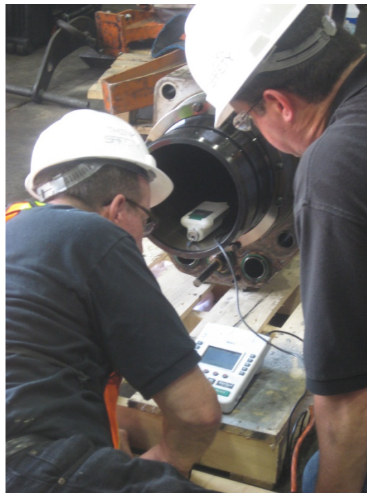
Figure 7: Chevron Oronite personnel measuring the surface area of 2R power assembly cylinder liner to categorize wear.
