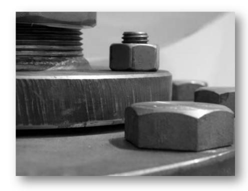
Tighten the manway bolts using the appropriate star pattern and company procedures.
