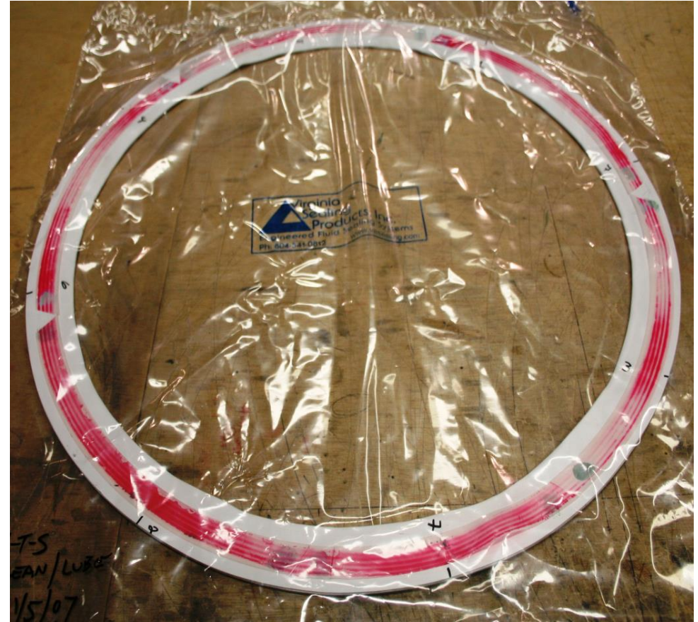
Cleaned & Lubricated Eyebolts More Uniform, Higher Overall Gasket Stress Developed
