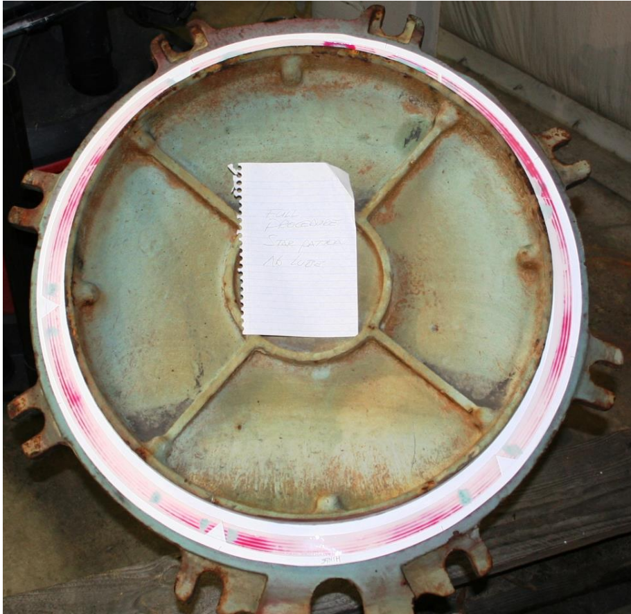
Unlubricated Eyebolts Non-Uniform, Lower Overall Gasket Stress
