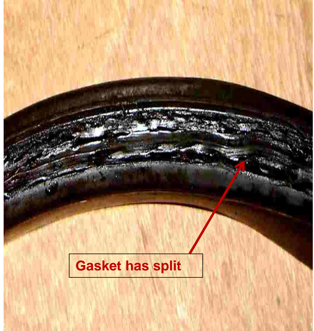
Viton® in Asphalt [Viton® 450°F, Asphalt = 400°F]
