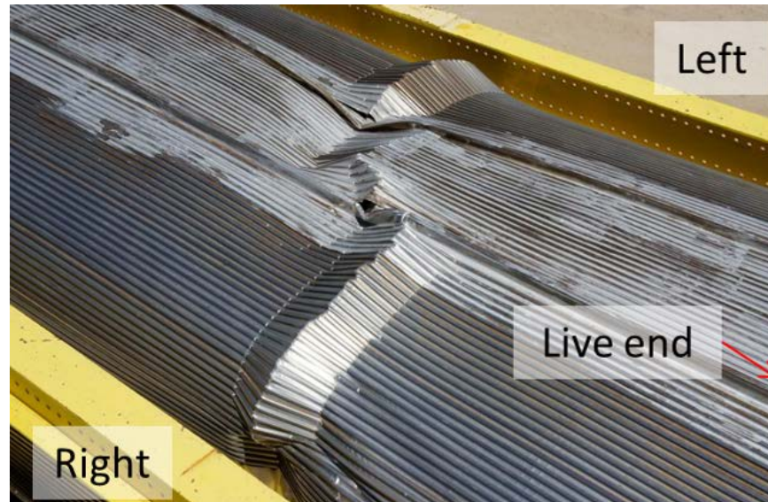
Figure 53. Buckled Roof, Car 248
