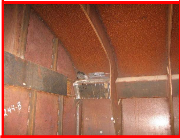
Figure 39. Strain Gage at Roof-Level Energy Absorber Support
