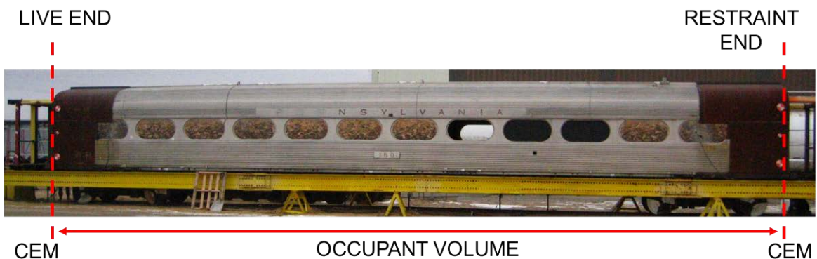
Figure 7. Car 244 in Test Frame, 800-kip Verification Test
