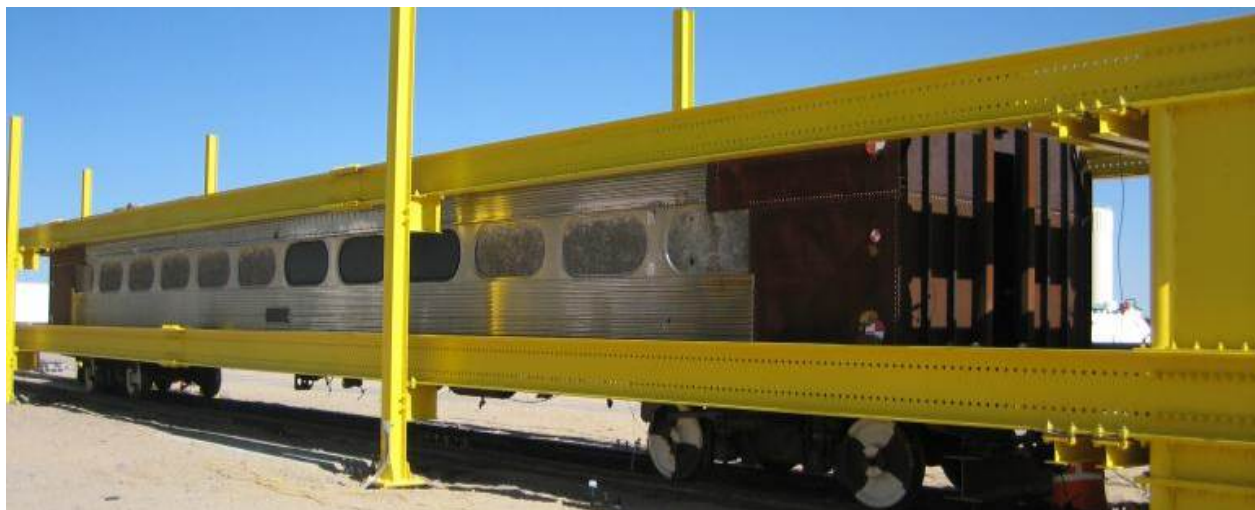
Figure 32. Car 248 in Test Frame, Crippling Test
