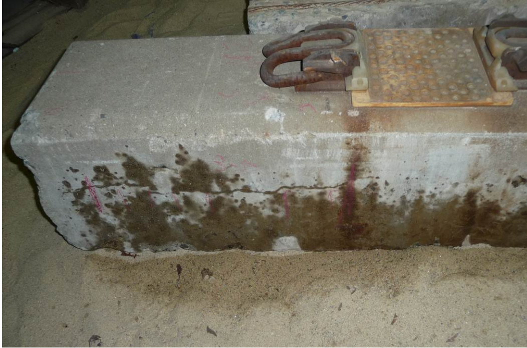
Figure 3.7. Photograph of one of the case study ties showing how the crack is revealed with the use of isopropyl alcohol.
