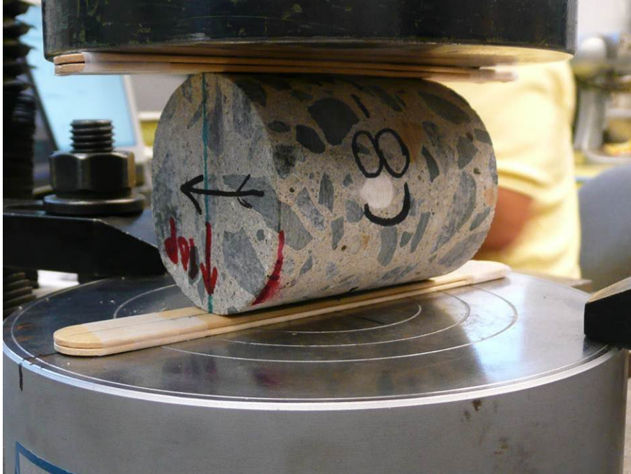
Figure 5.4. Tensile (splitting) test configuration.
