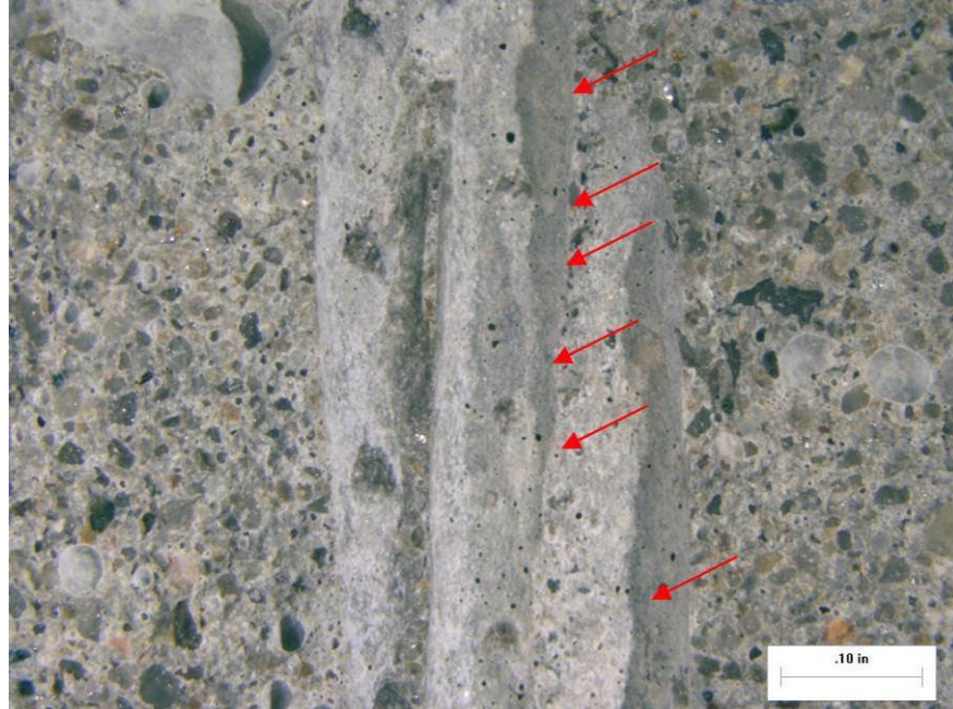
Figure 4.19. A magnified view of the polished cross-section in Core C17-3 showing the fracture surface just above the tendon. Red arrows point to the tear fractures in the fracture surface.
