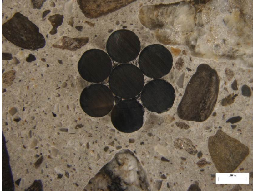
Figure 4.9. A magnified view of the polished cross-section in Core S1-3 showing a tight intimate bond between the tendon strands and the surrounding paste.
