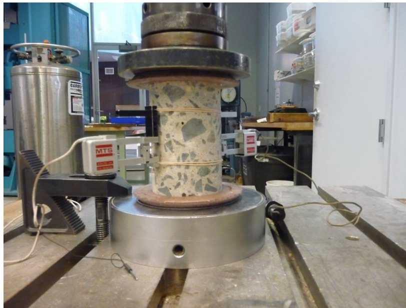
Figure 5.1. Set-up testing for the modulus of elasticity tests.
