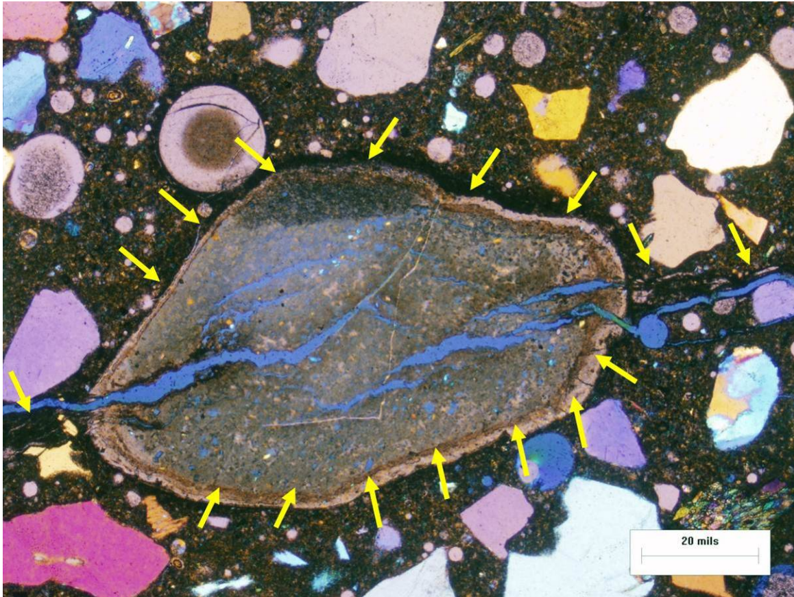
Figure 4.14. Magnified view of the microstructure in the body of Core C8-4 showing a reactive chert aggregate particle with ASR gel. Yellow arrows outline the reaction rim around the perimeter of the aggregate as well as the locations of ASR gel that partially fills cracks that extend outward from the aggregate and partially fills fractures in the surrounding paste structure.
