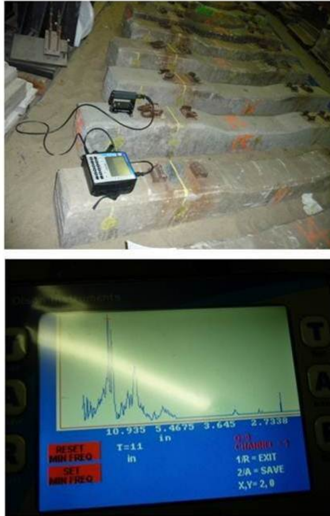
Figure 3.9. The impact echo device and a sample reading.
