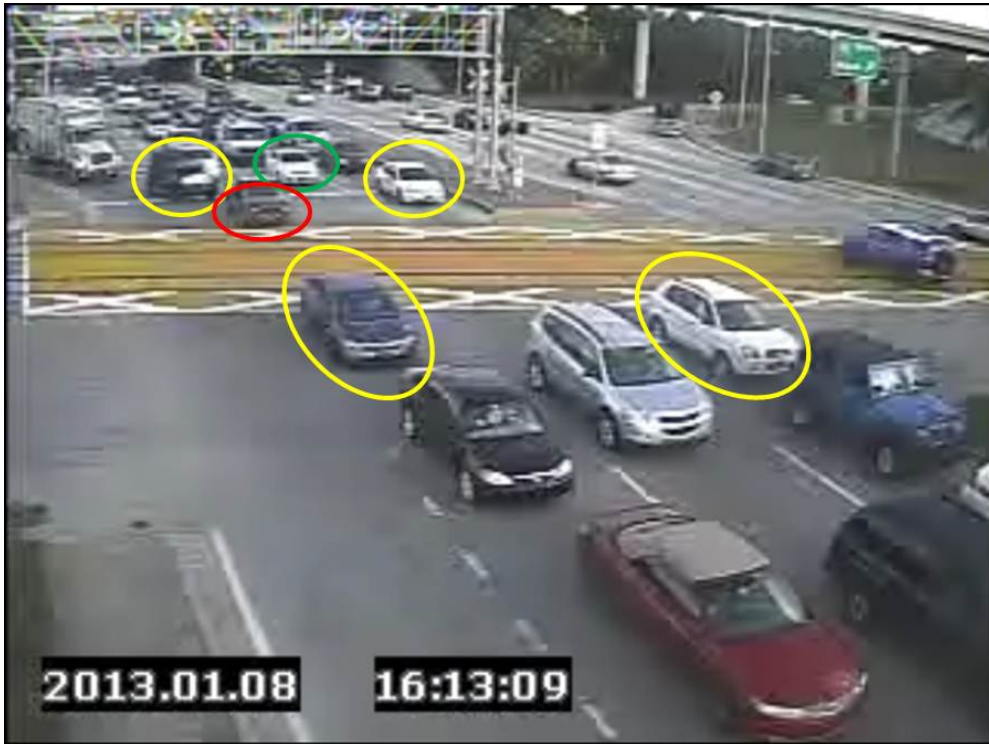
Figure A- 3. Many Westbound Vehicles Stopped on or Near the Tracks
