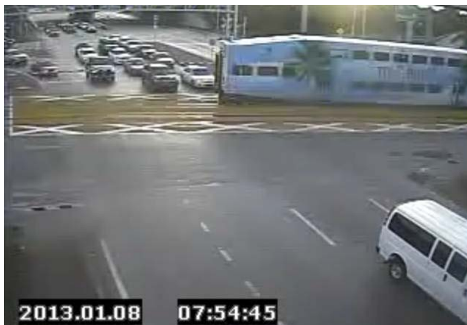
Figure 24. Westbound Vehicles Trapped Inside Gates during an Activation
