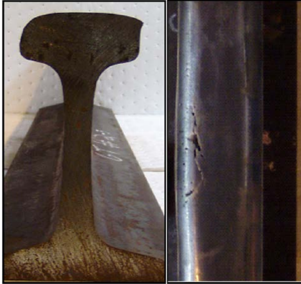
Figure 6. Rail with Worn Geometry Characteristics and Surface Flaws
