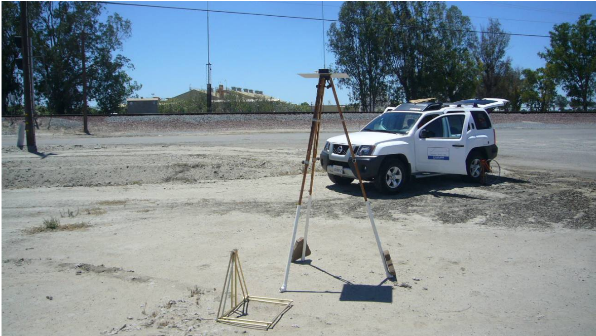
Figure 3.5-A-1 RF measurement equipment: A.H. Systems monopole antenna
