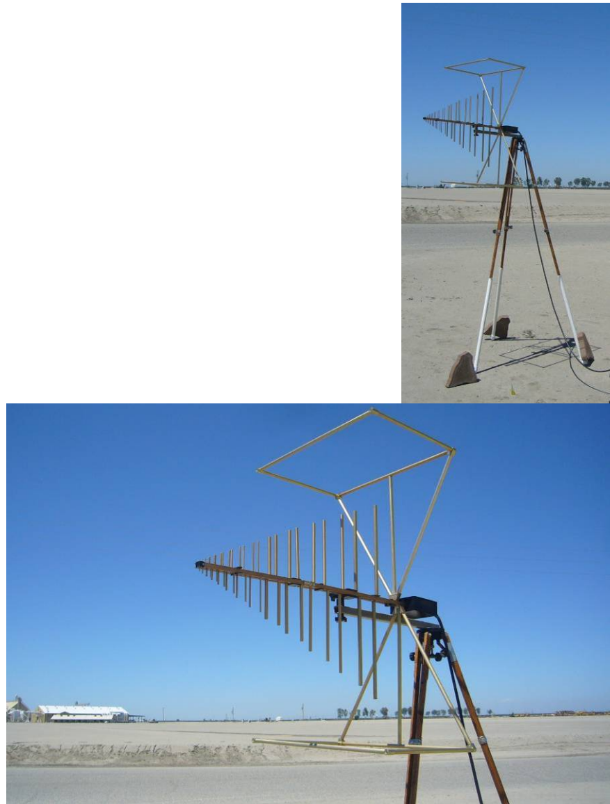
Figure 3.5-A-2 RF measurement equipment: A.H. Systems bi-logical antenna
