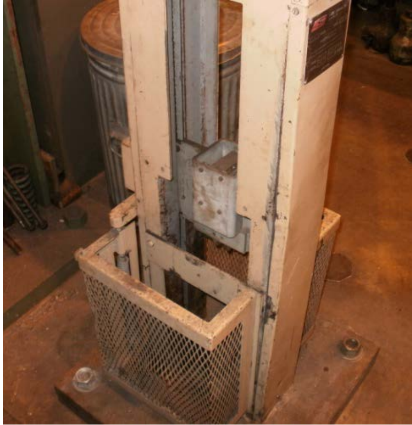
Figure 29. Drop load fixture showing opening at bottom and vertical drop load.
