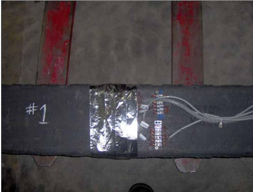
Figure 2. Example of strain gage wiring at the tie center. The strain gages were protected under tape, with the wires leading to the end of the tie to allow data collection.
