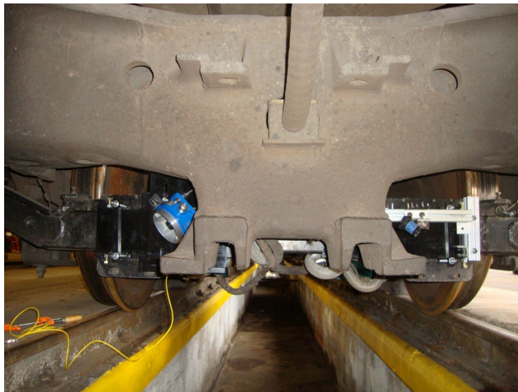
Figure 42: Truck mounted LIDAR lenses, pointing at gauge corner
