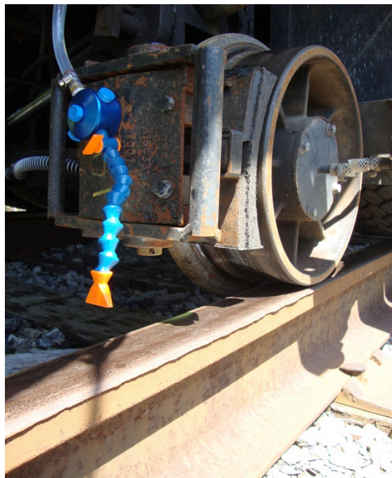
Figure 7: Water-dispensing system used to wet the rail attached to R4
