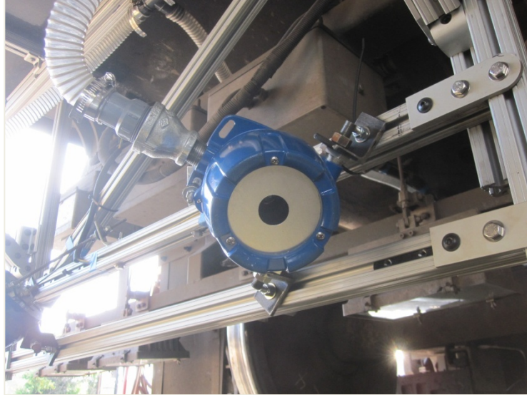
Figure 58: LIDAR lens housing attached to an air supply to create positive air pressure inside the housing
