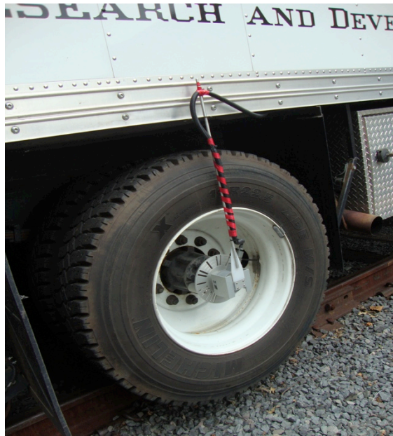
Figure 6: Encoder attached to the right rear (passenger side) truck axle
