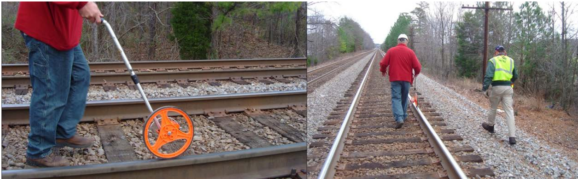
Figure 26: 1000 ft being walked out for ground-truth calibration run
