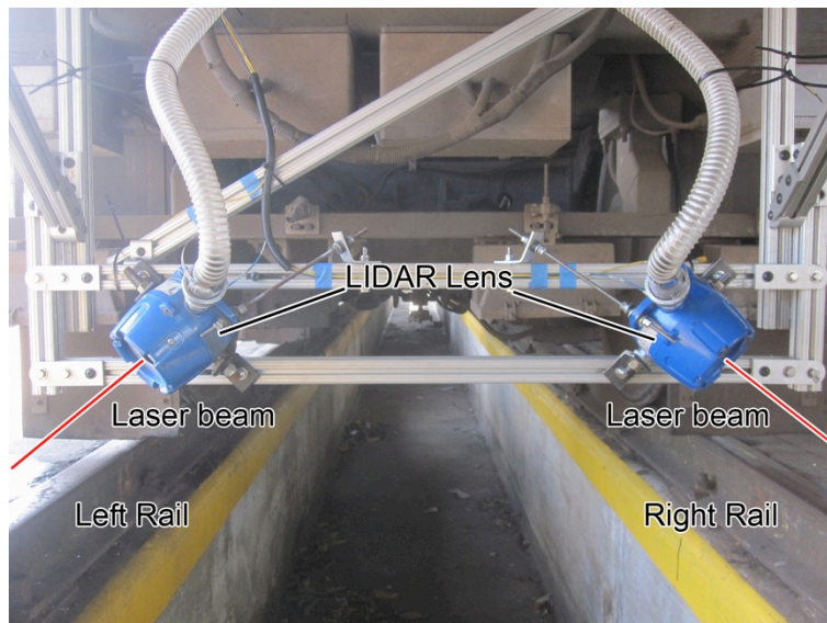
Figure 57: Body-mounted LIDAR system onboard the track geometry car with the gauge corner beam alignment
