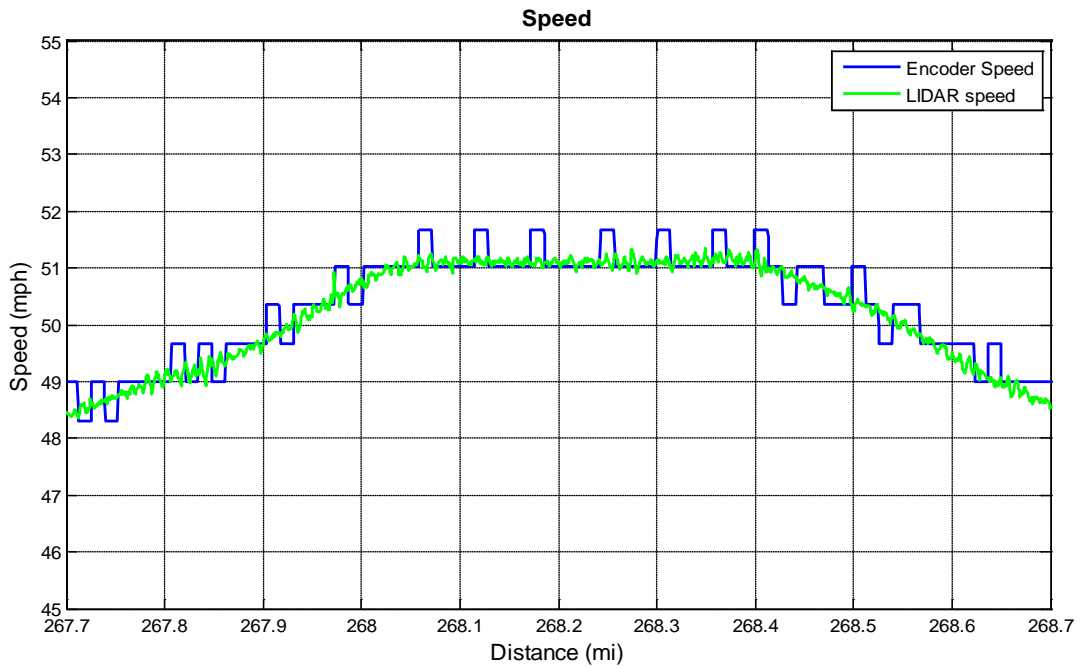
Figure 60: A close-up of encoder and LIDAR speed measurements from 1 mile of revenue service track
