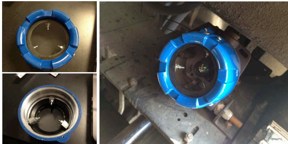
Figure 45: Explosion-proof protective housing securing the LIDAR lenses onboard the track geometry car
