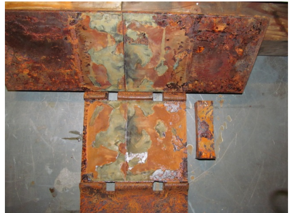
Fig. A-2. Week 1 – PD after Humidity
