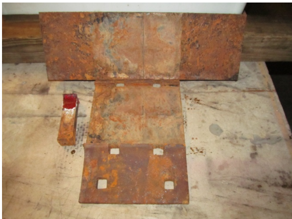
Fig. A-11. Week 3 – ALL after Salt Water
