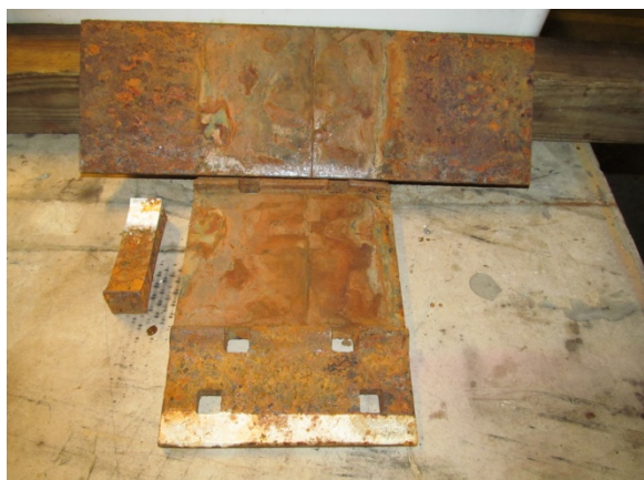
Fig. A-5. Week 3 – PD after Salt Water
