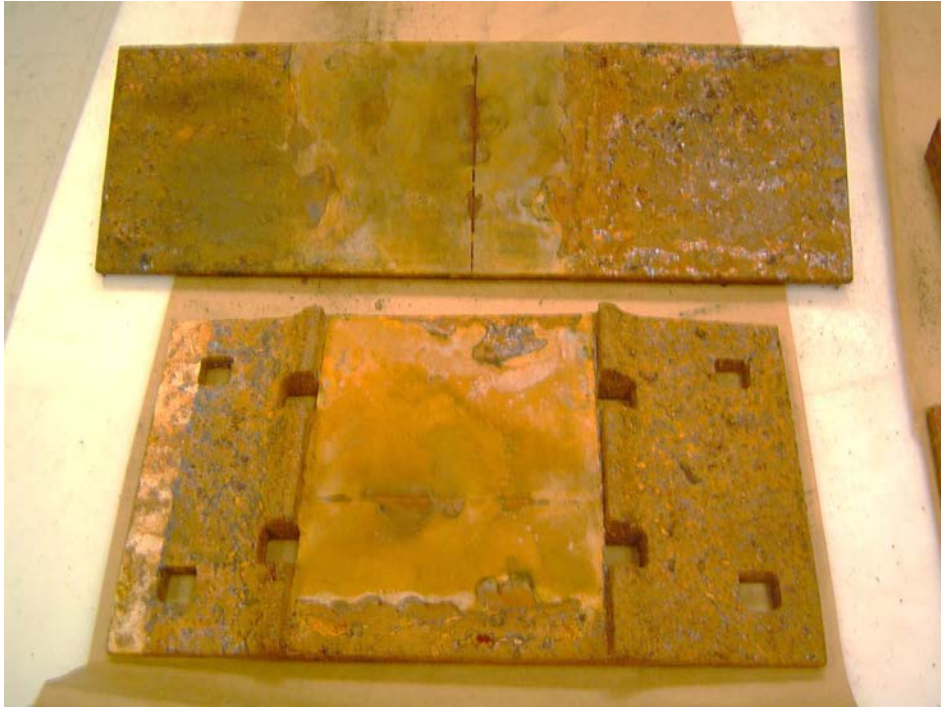
Figure 30. PD Treated Samples after 3-Week Exposure (Tie Plate and Flange Bottom)
