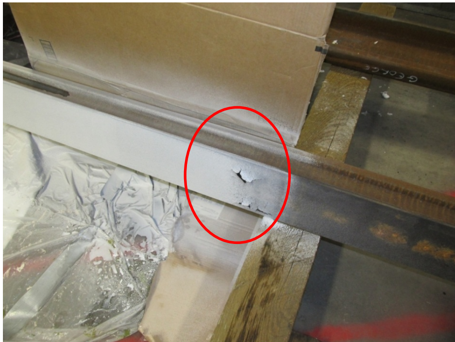
Figure 15. EonCoat® Sprayed Rail Segment
