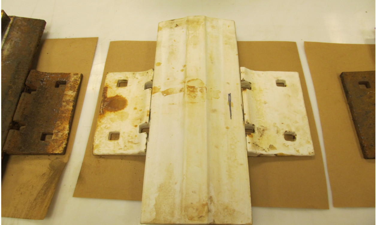
Figure A-27. EonCoat® after Cleaning
