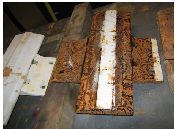
Fig. A-4. Week 2 – PD after Humidity
