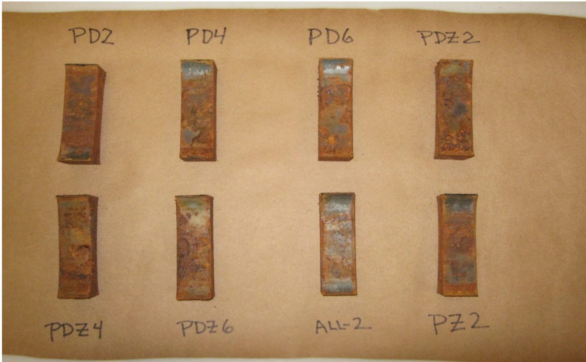
Figure 16. Bottoms of Samples after 2-Week Corrosion Cycle
