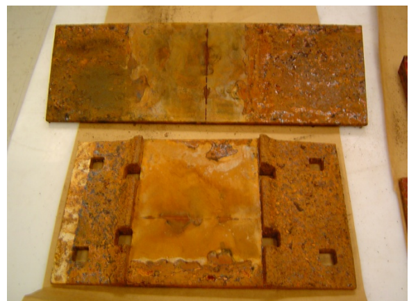
Fig. A-6. Week 3 – PD after Humidity
