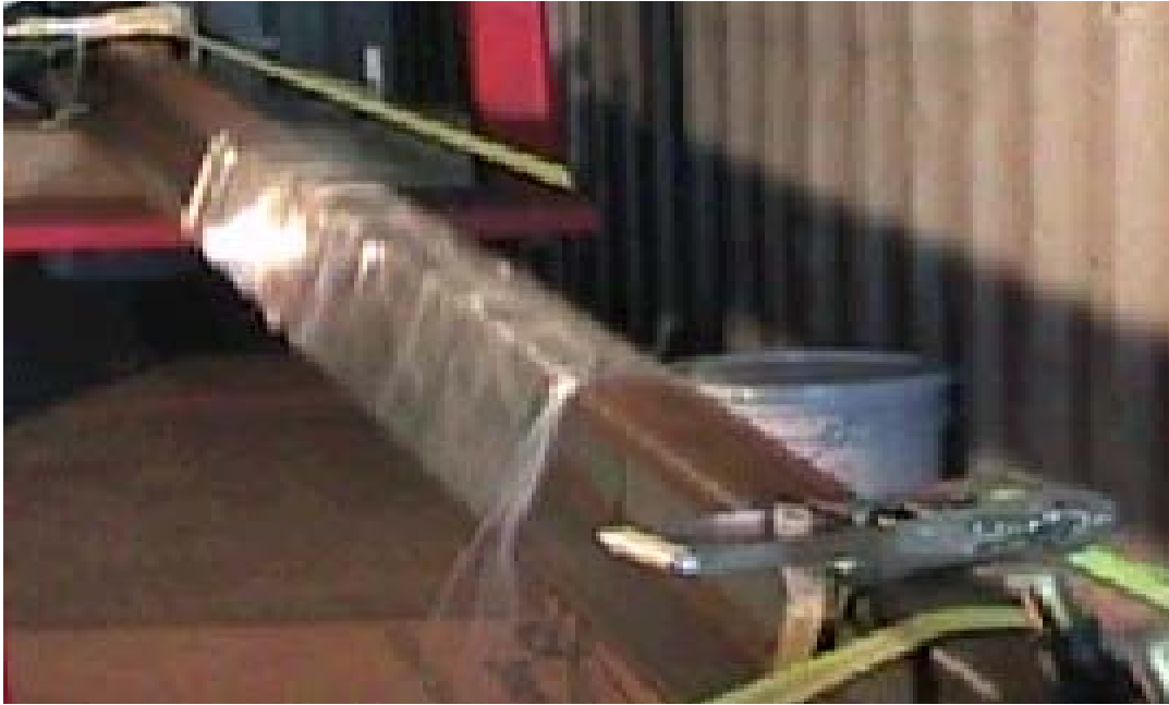
Figure 12. Rail Suspended in Resonant Fatigue Apparatus
