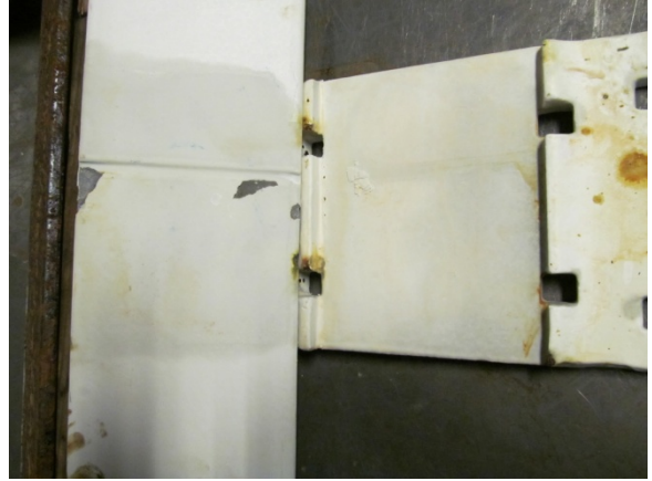
Fig. A-14. Week 1 – EC after Humidity
