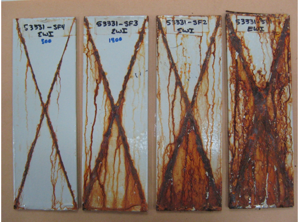
Figure B-4. EWI, Scribed to Metal. L→R: 500, 1500, 3000, 5000 Hours
