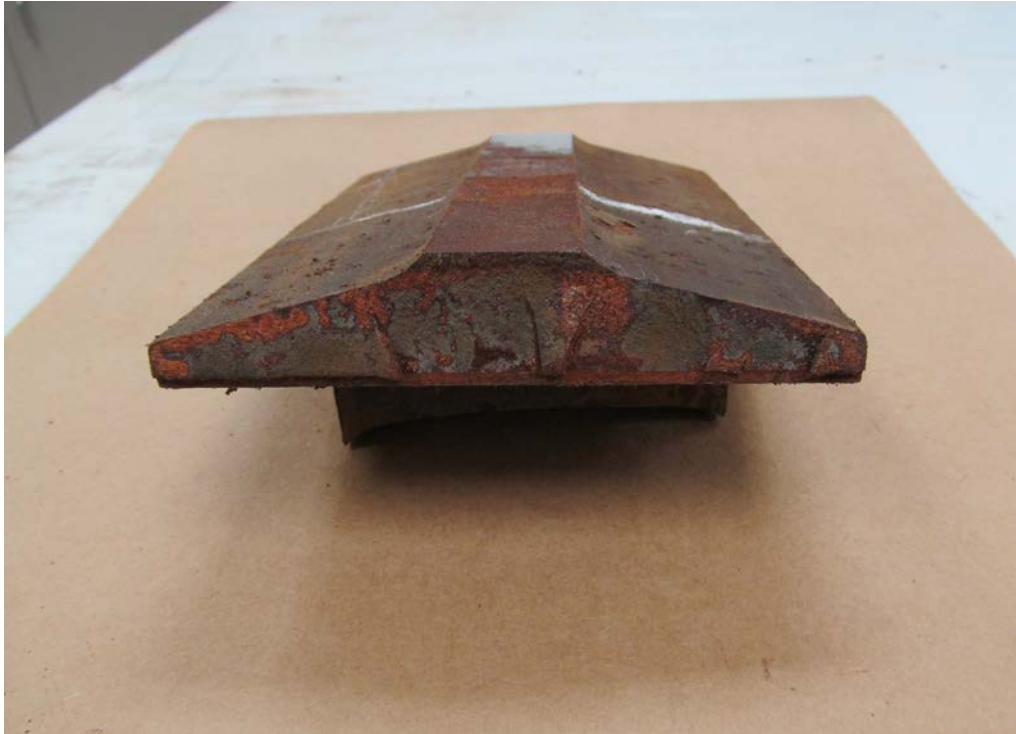
Figure 36. Fracture Surface of Corroded Sample with No Protection
