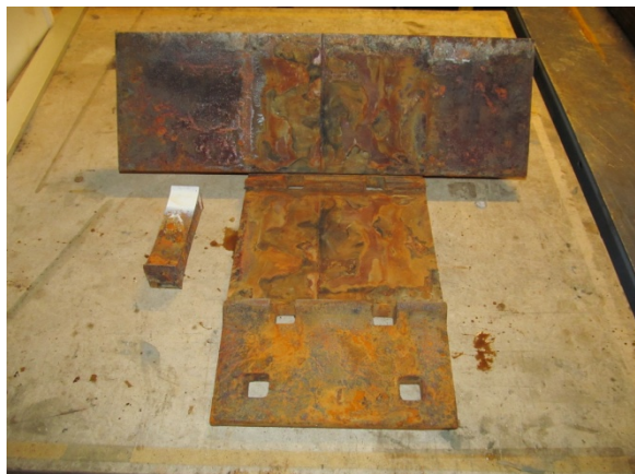
Fig. A-3. Week 2 – PD after Salt Water
