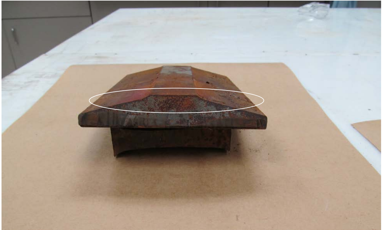
Figure 41. Fracture Surface of Corroded Sample with ALL Treatment
