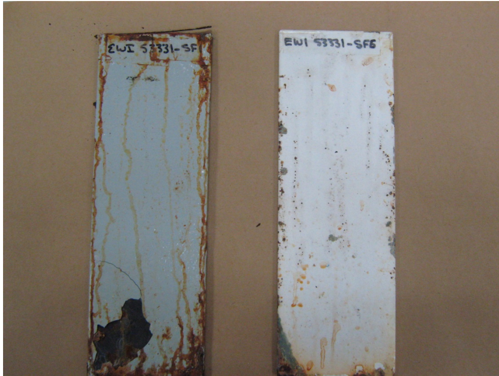
Figure B-3. EWI (left) and EonCoat® (right) after 5,000 Hours, Back Side
