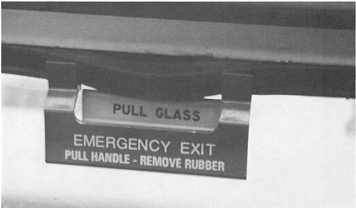
Close-up of Interior Emergency Window Exit Handle
