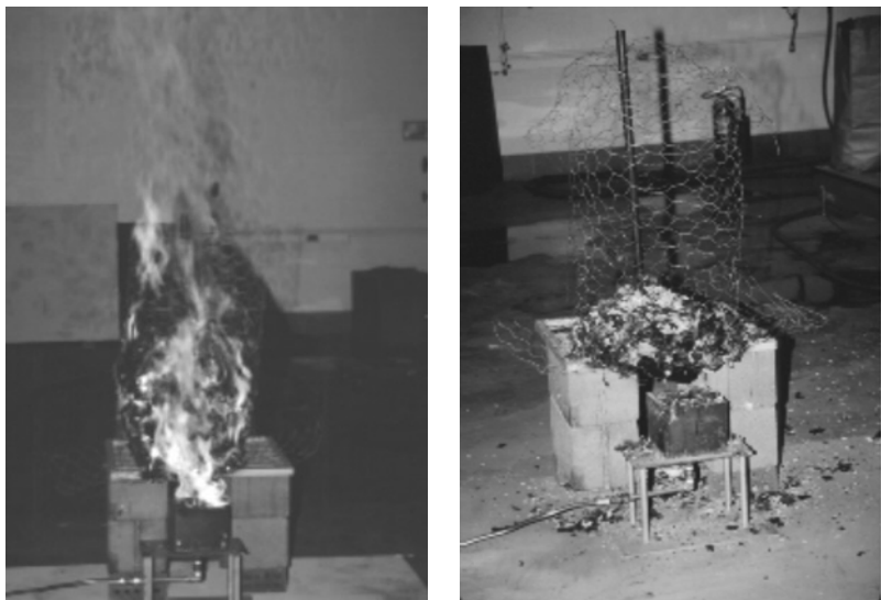
Figure A-18. Trash Bag Test - During and After Gas Sand Burner Ignition
