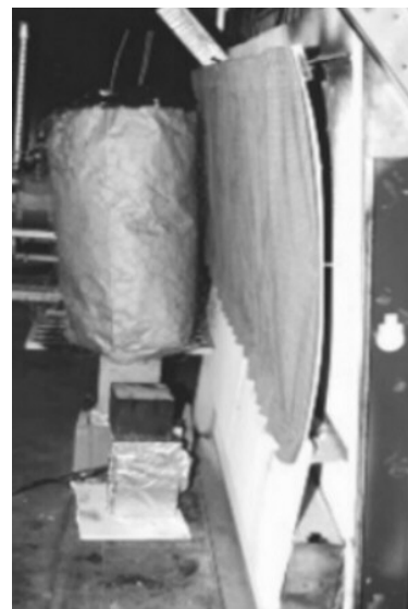
Figure A-17. Window and Drape Tests - Trash Bag/Gas Sand Burner Ignition Source
