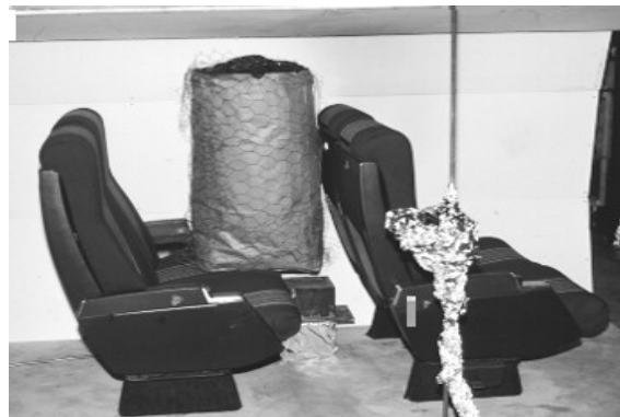
Figure A-6. Coach Seat Assembly Test - Trash Bag/Gas Sand Burner Ignition Source
