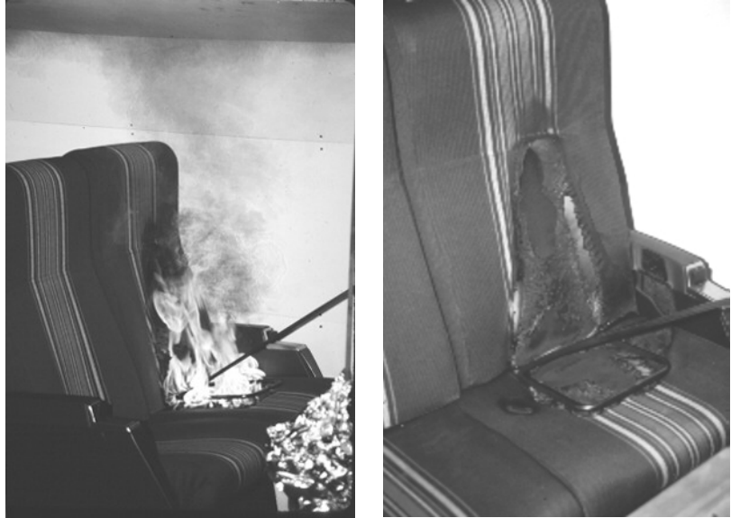
Figure A-22. Seat Assembly Test - During and After TB 133 Burner Ignition
