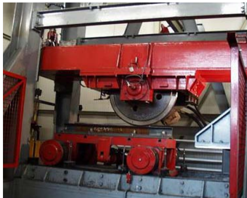
Figure 14. Single wheel test rig shown as an example of layout
