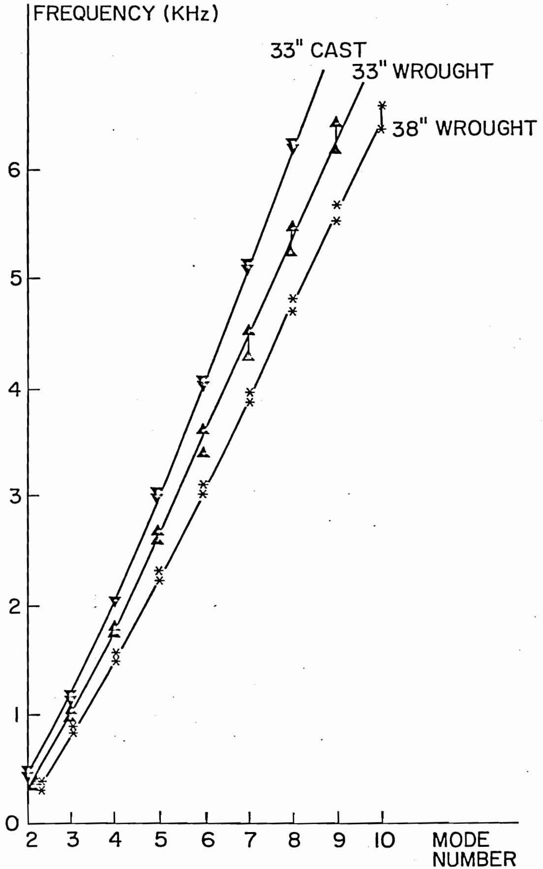
FIGURE 1.5 A.S.I. - MODE SEARCH : MODAL FREQUENCY VS. MODAL NUMBER FOR DIFFERENT WHEEL TYPES.
