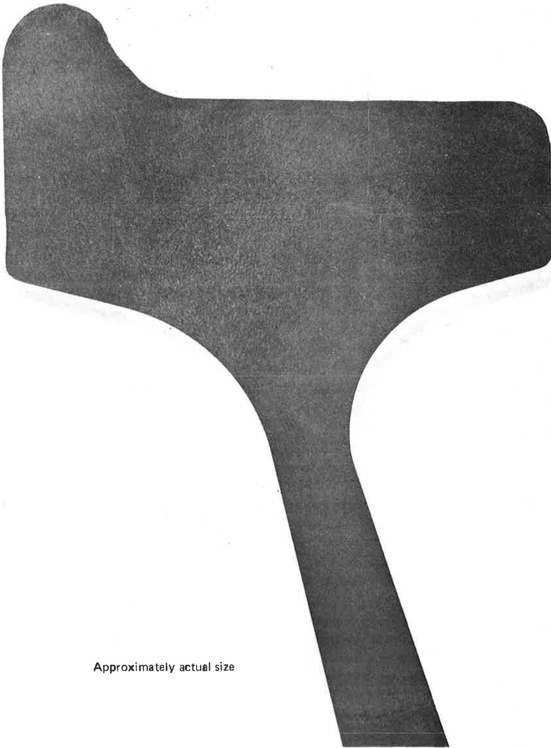
FIGURE 36.—MACROSECTION OF CLASS SUB A WHEEL (WHEEL 8), GRAIN FLOW SECTION GF2 (METROLINER TYPE WHEEL)
