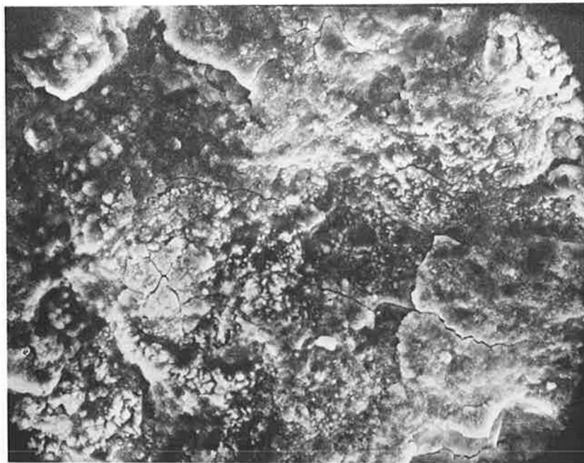
FIGURE 58.—SCANNING ELECTRON MICROGRAPH OF SPECIMEN 44-F4 TAKEN FROM CLASS A WHEEL, TESTED IN 3.5% NaCl AQUEOUS SOLUTION
