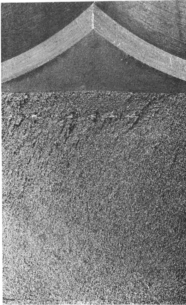
FIGURE 50.—FRACTURE OF COMPACT SPECIMEN FFE-KC4 TAKEN FROM GRADE F AXLE AND TESTED AT -40° F
