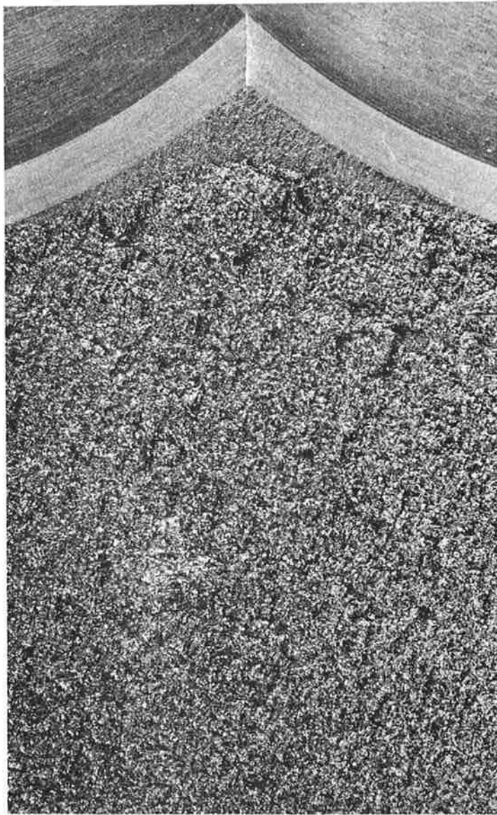
FIGURE 48.—FRACTURE OF COMPACT SPECIMEN UUE-KC4 TAKEN FROM GRADE U AXLE AND TESTED AT -40° F
