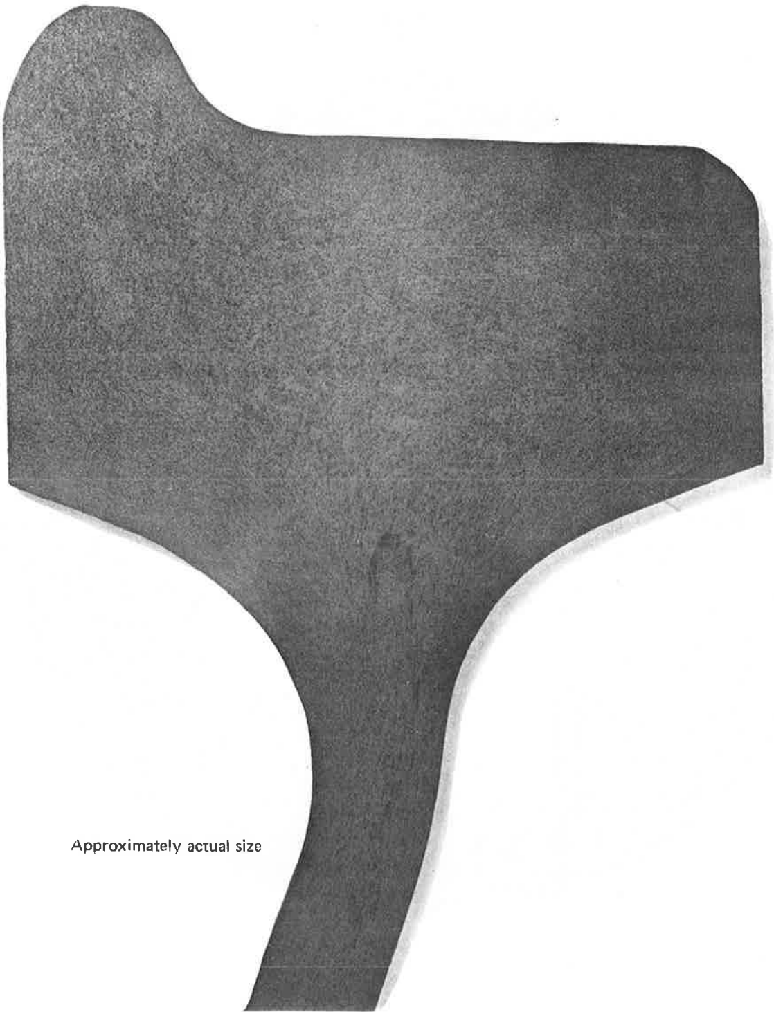
FIGURE 37.—MACROSECTION OF CLASS B WHEEL (WHEEL 9), GRAIN FLOW SECTION GF5
