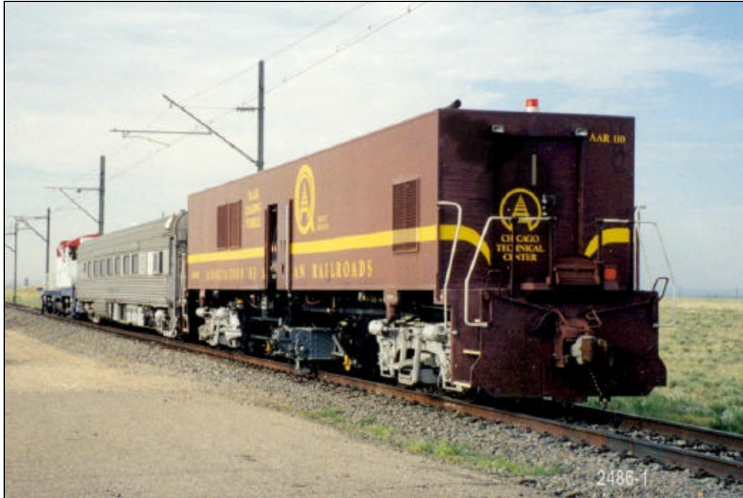
Figure 4. TTCI's Track Loading Vehicle (TLV), Test Car, and Locomotive Consist. (The TLV measures gage strength, lateral track stability, and vertical track stiffness on the move.)
