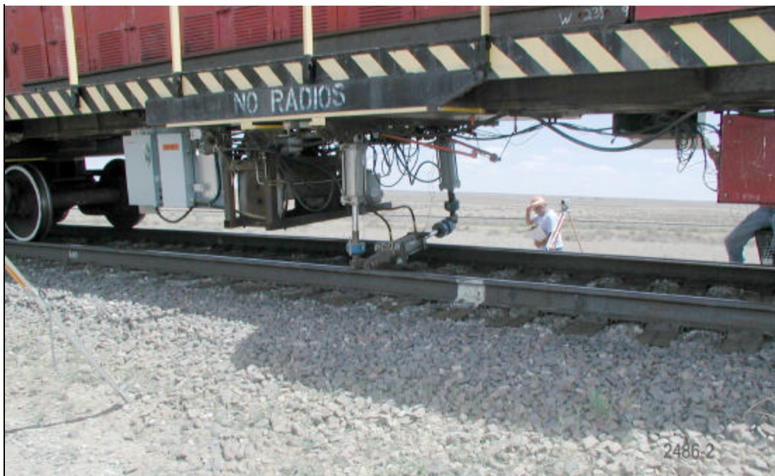
Figure 3. TTCI's Rail Force Calibration 605 Car Deploying its Hydraulic System
