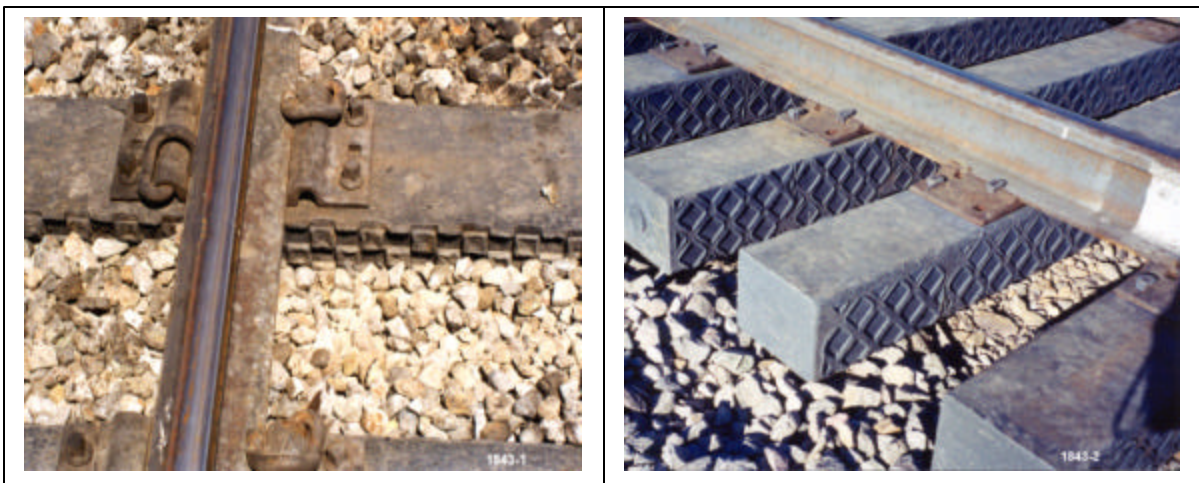
Figure 1. (Left side) USPL ® Plastic Tie Test Zone with Elastic Fasteners in the 5-degree Curve; (Right side) TieTek ® Plastic Tie Test Zone in the 6-degree Curve with Cut Spikes
