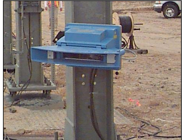
Figure 5. System 2 Vehicle/Obstacle Detection Sensor, Combined Low Power Laser and Video Imaging System
