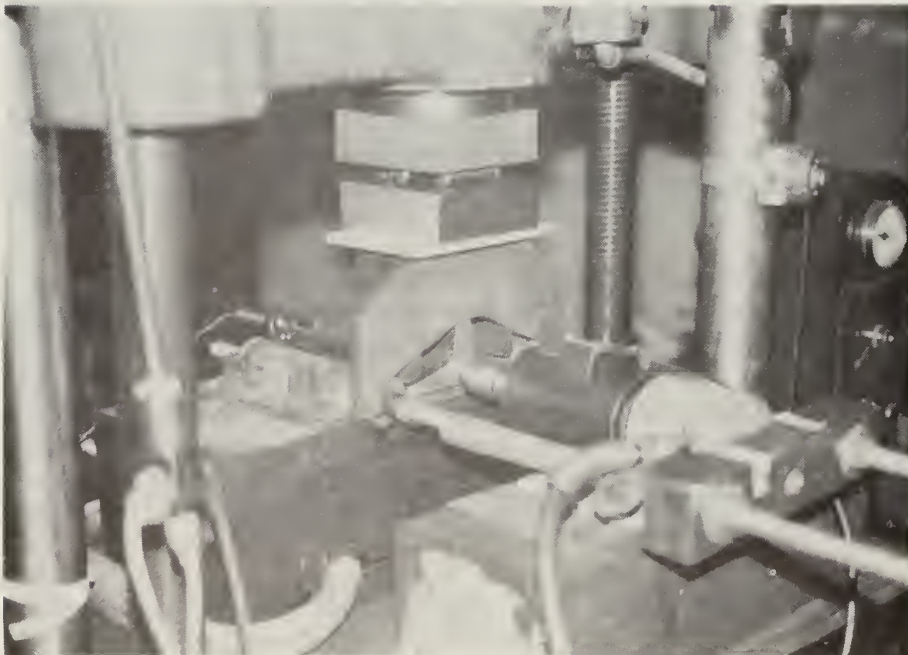
(b) Toe Load Provided by Test Machine
