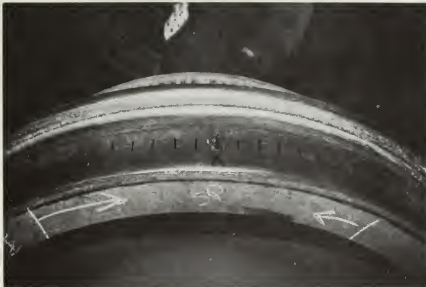
(b) Worst-Case Flattened Wheel Condition
