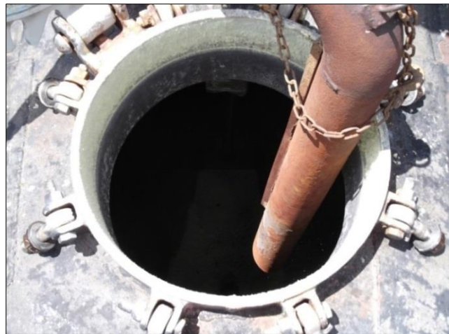
Figure 13: Loading a Rail Tank Car
