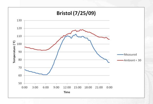
Empirical model used by industry does not provide information on how rail temperatures change throughout an entire day
