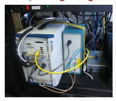
The KVM network used to interface with the PXI hardware
