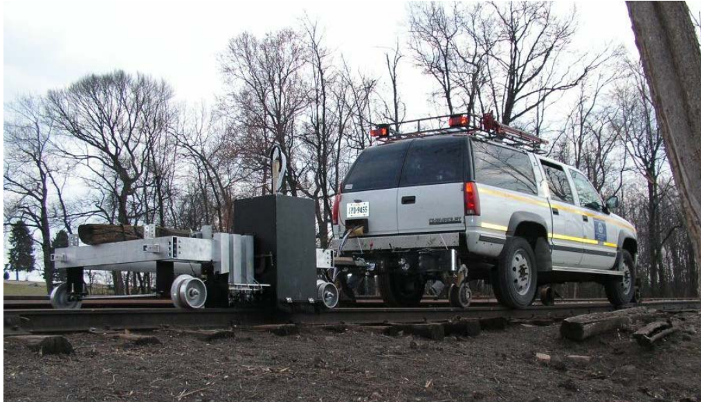
Figure 4.9. The Inspection Prototype Towed by the FRA Hy-Railer Managed by ENSCO during the First Field Test
