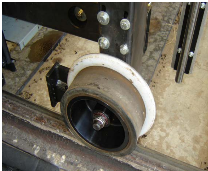
Figure 9.4. Detail of the New Nylon Wheel Flanges Required for Noise Reduction
