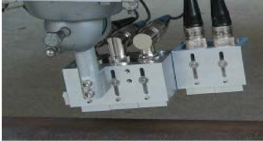
Figure 6.2. Piezocomposite Sensors Arranged in an Array Configuration
