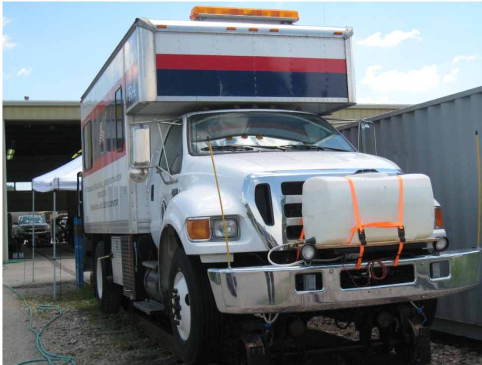
Figure 10.1. Water Reservoir for the Supply of the Water Spray System Installed to Reduce the Noise Created at the Wheel-Rail Interface
