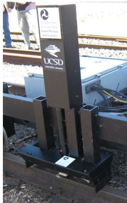
Figure 6.3. (left) Water-Tight Steel Case Containing All Electronic Components Attached to the Sensing Lines; (right) Improved Covers for Laser and Sensors
