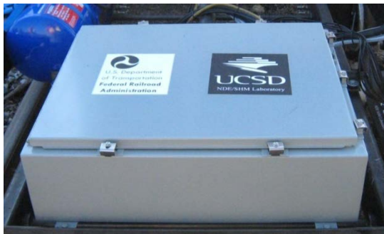
Figure 6.3. (left) Water-Tight Steel Case Containing All Electronic Components Attached to the Sensing Lines; (right) Improved Covers for Laser and Sensors
