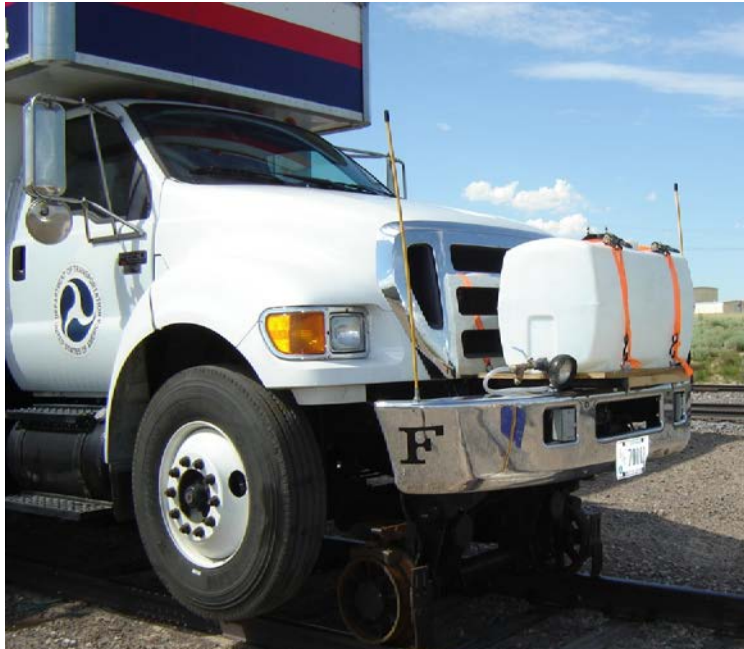
Figure 9.5. The 50-Gallon Water Tank for the Water Spray System Mounted on the Front of R-4
