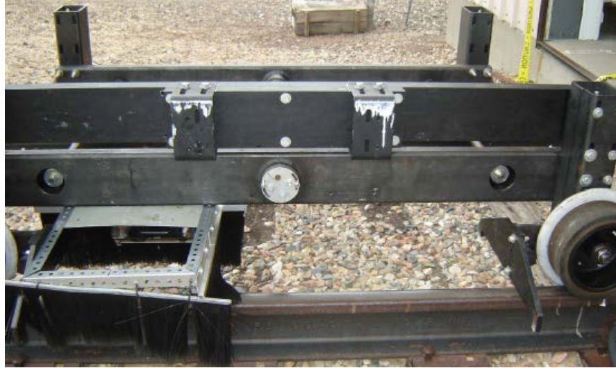
Figure 9.3. ENSCO Laser Positioning Sensor Mounted on the Cart Beam
