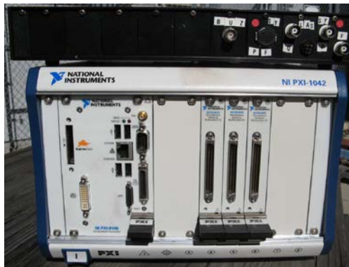
Figure 7.1. Breakout Box and PXI Unit; the Box Is Connecting the Sensor Lines to the PXI Data Acquisition Unit
