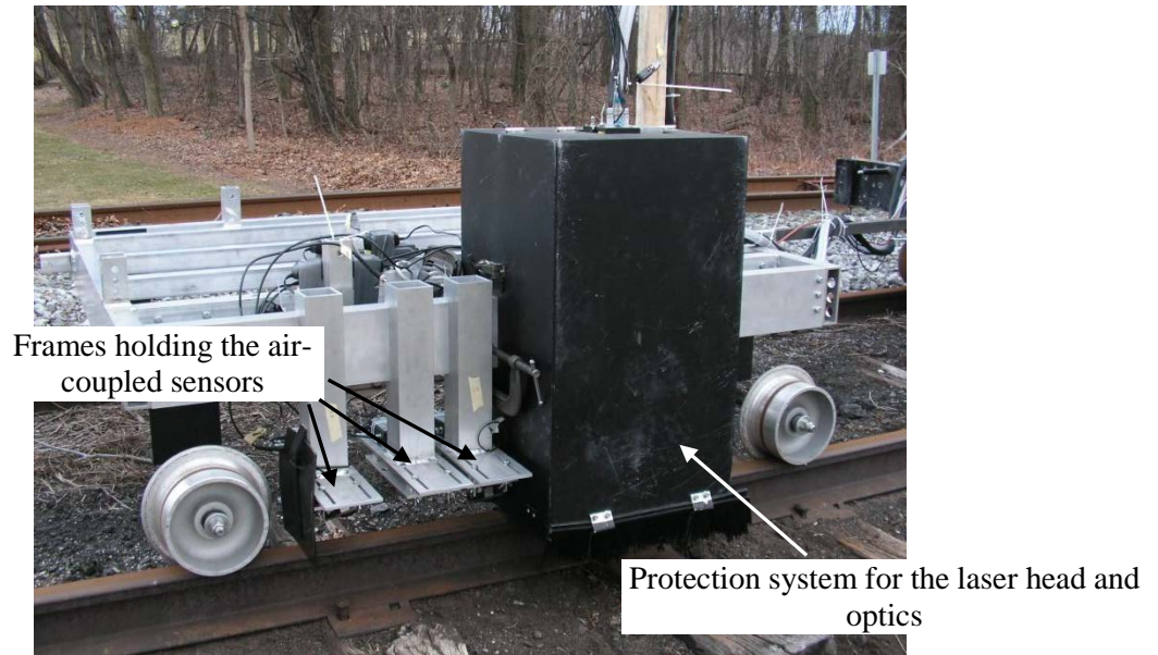
Figure 4.6. Laser Head and Sensors on ENSCO's Cart during First Field Tests
