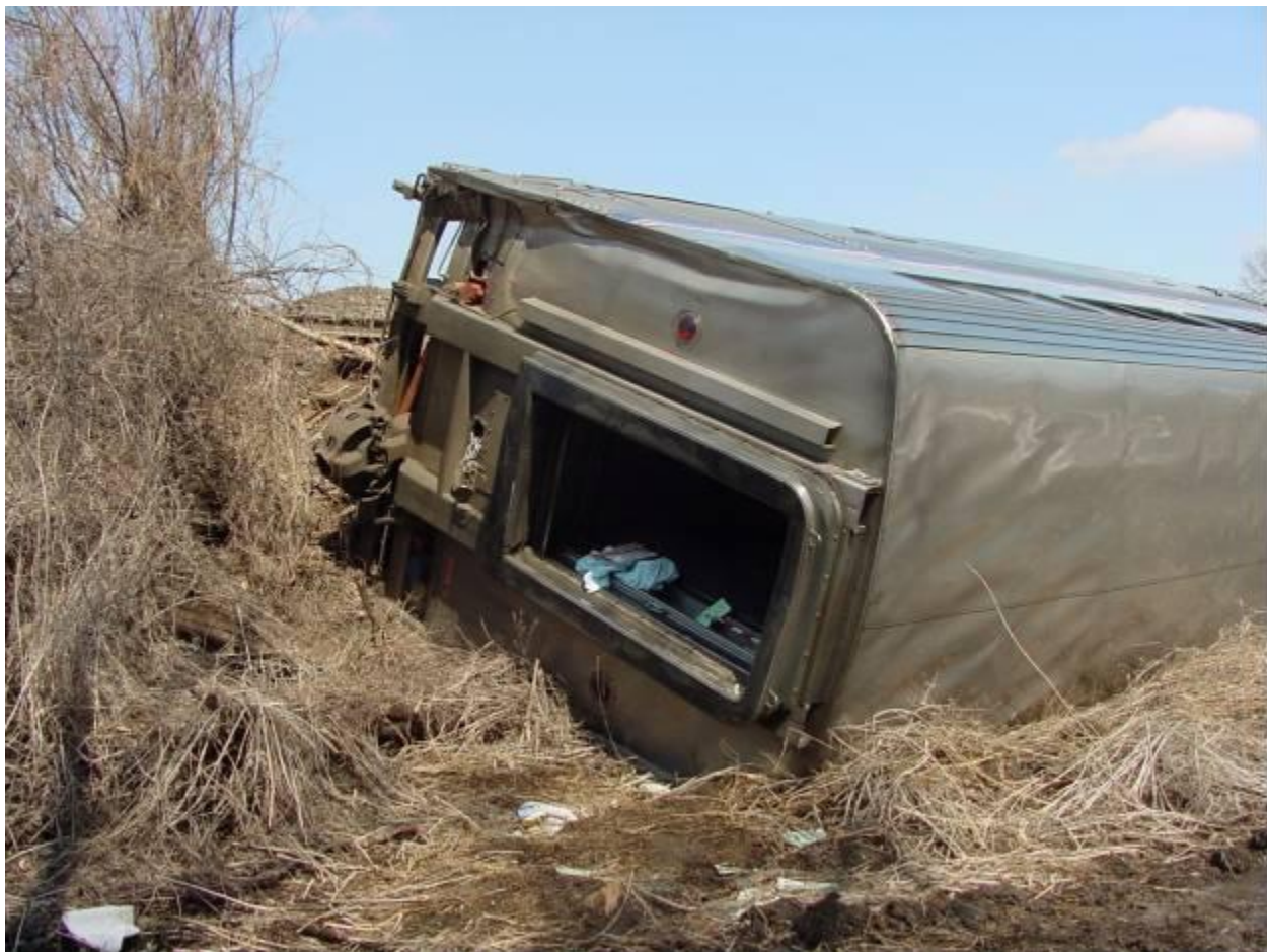
Figure 37. Derailed Car Supported by its Roof and Side Structures (Nodaway, IA – 2001)
