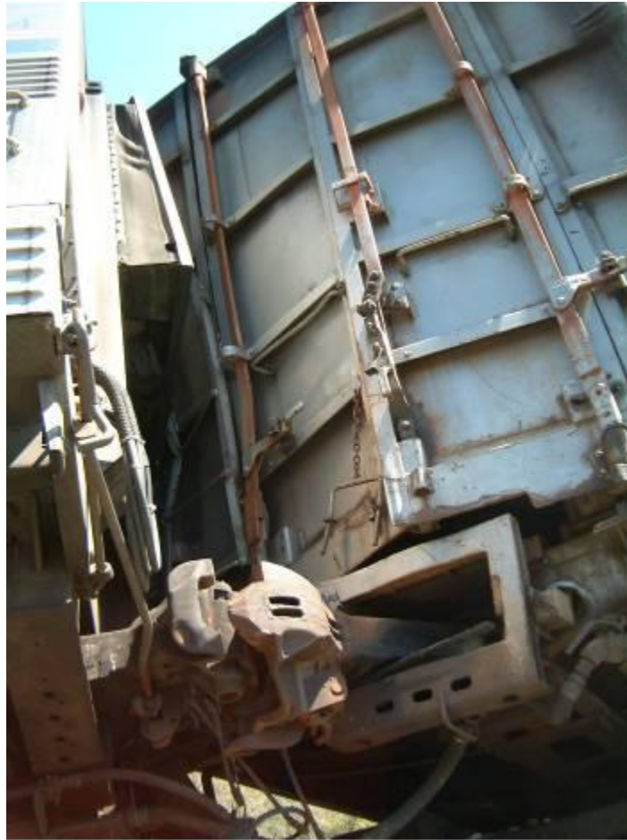
Figure A10. Coupler between the Last Passenger Car and the First Auto Car
