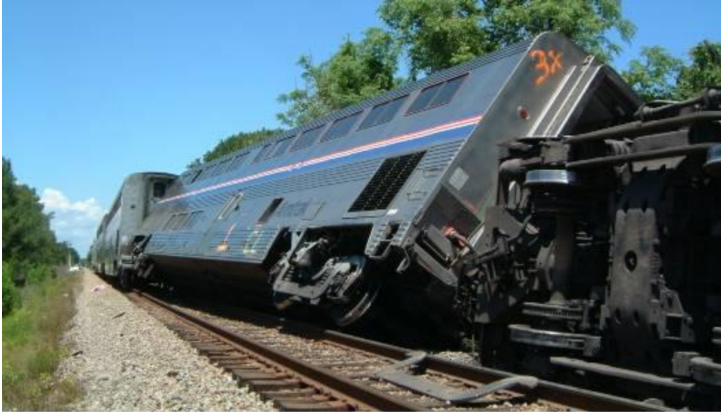
Figure A6. View of First Derailed Passenger Car Looking toward Lead End of Train
