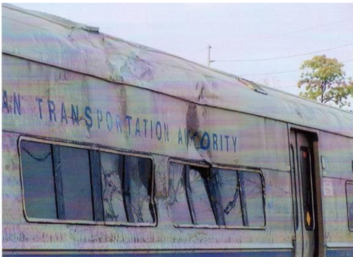
Figure 36. MU Side Structure Damage after Striking Construction Equipment (Hewlett, NY – 2001)
