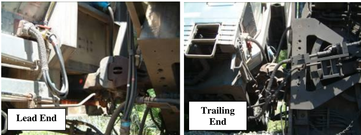
Figure A7. Closeup Views of the Couplers of the First Derailed Passenger Car
