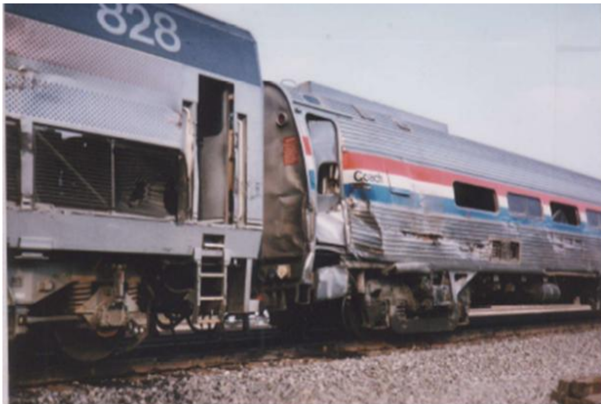
Figure 35. Corner and Side Damage to Trailing Coach (Gary, IN – 1997)
