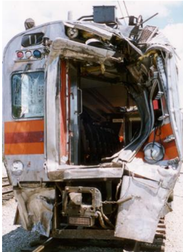
Figure 34. Lead Cab Car after Striking Truck at Highway-Rail Grade Crossing (Portage, IN – 1998)
