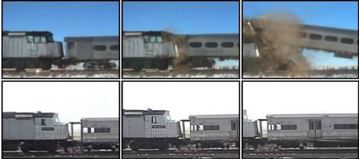
Figure 4. Frames from High-Speed Movies of Conventional (top) and CEM (bottom) Train-to-Train Tests
