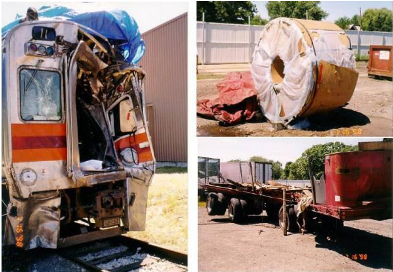
Figure A3. Postcollision Photographs of Cab Car, Truck Trailer, and Steel Coil Involved in Portage, IN, Grade Crossing Collision
