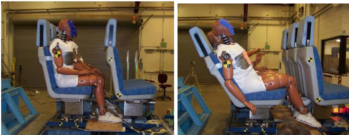
Figure 14. Pre- and Posttest Photos of Rear-Facing 12g Sled Test
