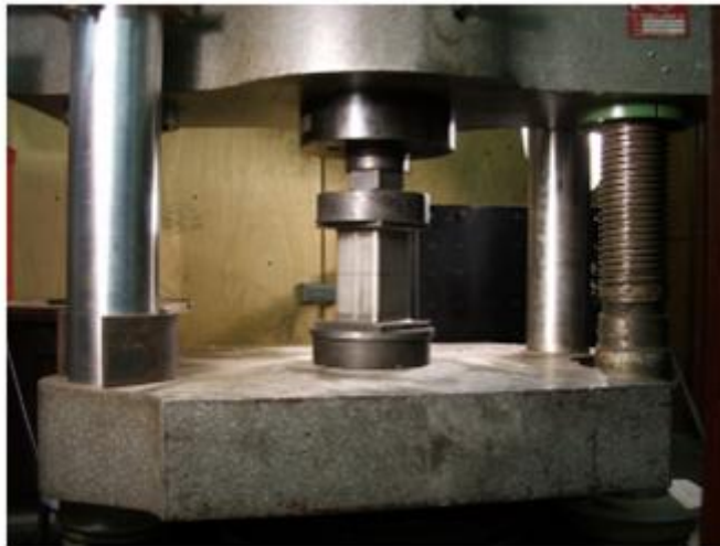
Figure 83. Example of a Quasi-Static Test of a CEM Component
