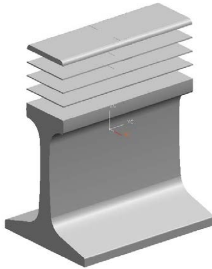
Figure 1. Drawing of Railhead and Locations of Typical Slices for Tests
