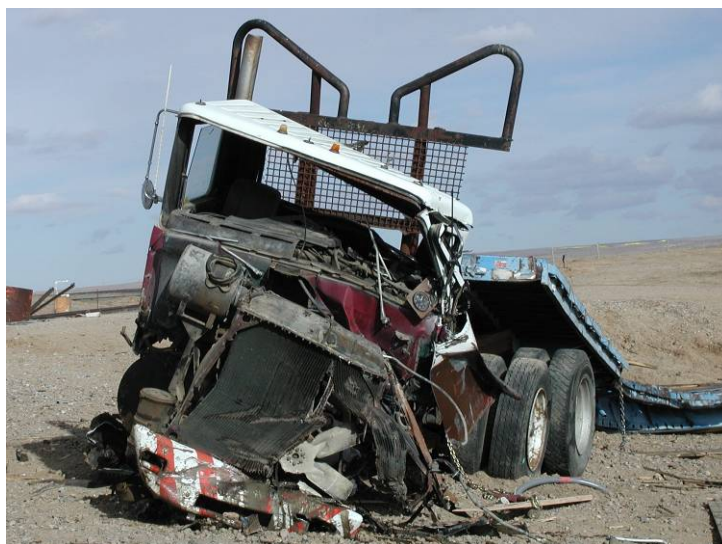
Figure 10. Stationary Vehicle at Grade Crossing after Test Collision
