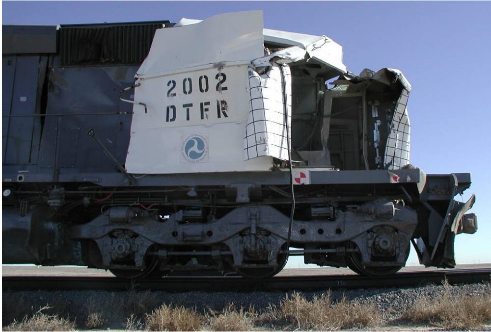
Figure 11. Damage to Locomotive after Collision
