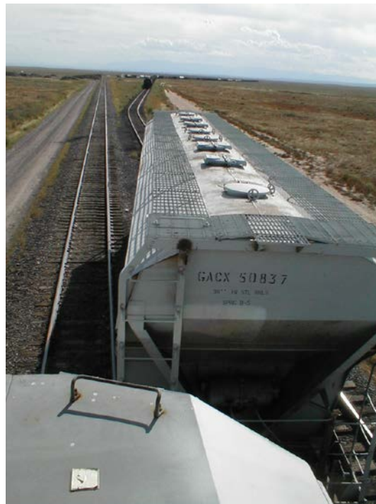
Figure 8. Alignment of Locomotive and Covered Hopper Car at Point of Impact
