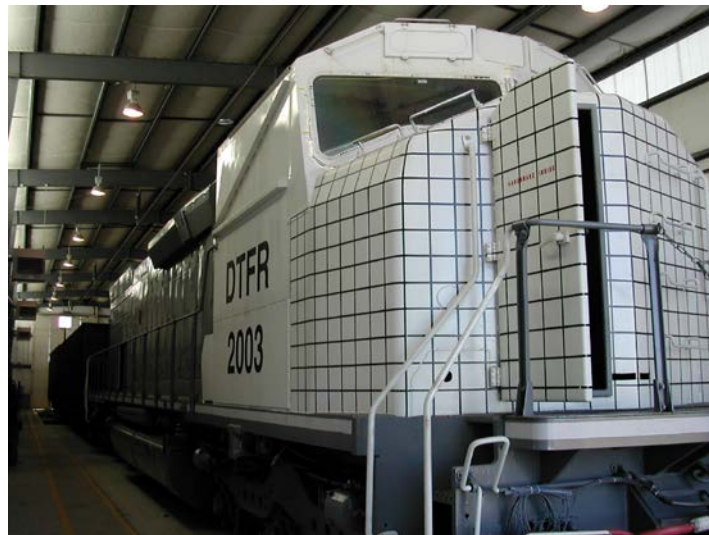
Figure 6. Locomotive and Bullet Consist before Impact Test
