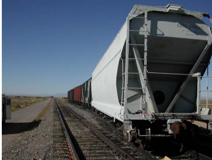
Figure 7. Covered Hopper Car and Target Consist before Impact Test
