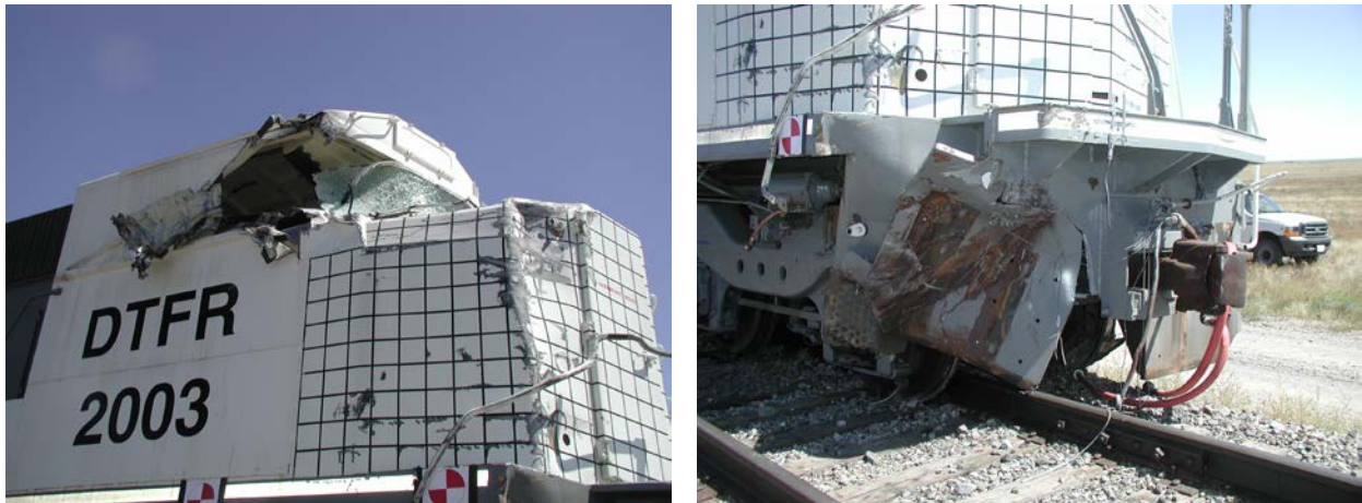
Figure 16. Damage to Locomotive
