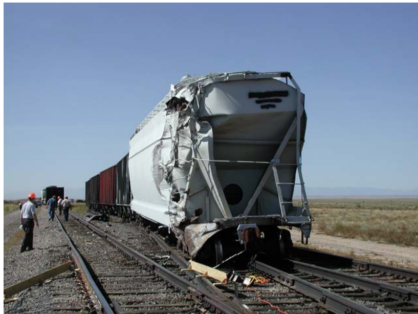
Figure 17. Covered Hopper Car after Collision
