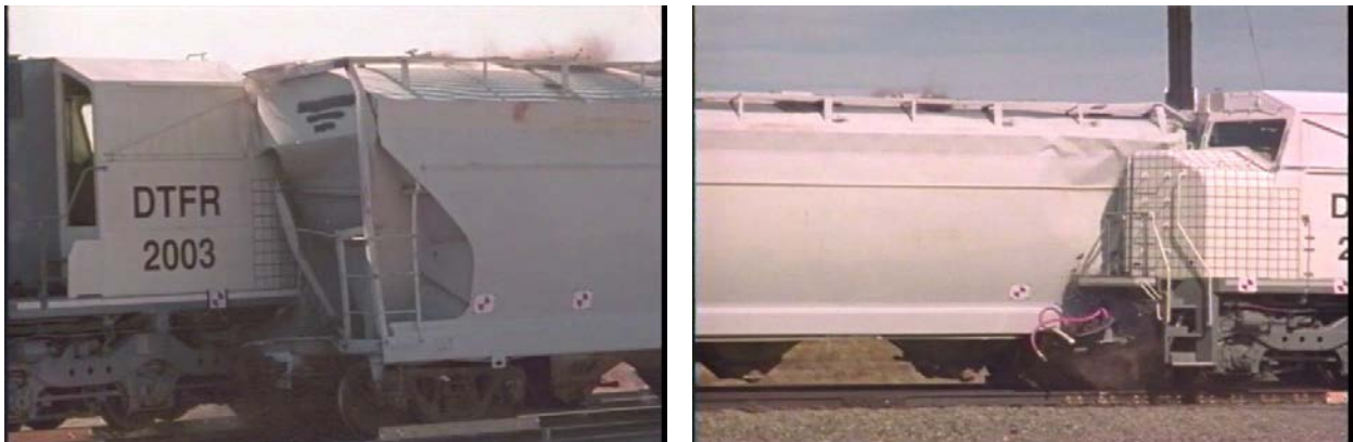
Figure 13. Hopper Stiff Corner Contacts Windshield Corner Post
