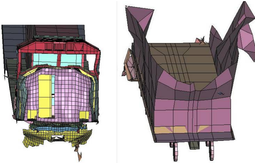
Figure 23. Locomotive and Hopper Car Damage from Simulation
