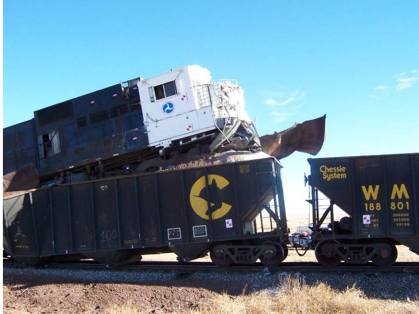
Figure 19. Hopper Car after Collision
