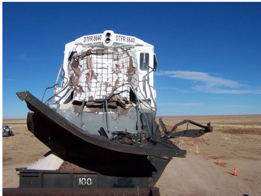
Figure 18. Damage to Locomotive
