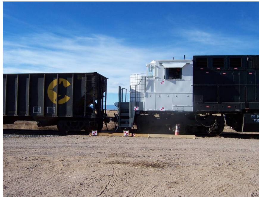
Figure 9. Alignment of Locomotive and Covered Hopper Car at Point of Impact
